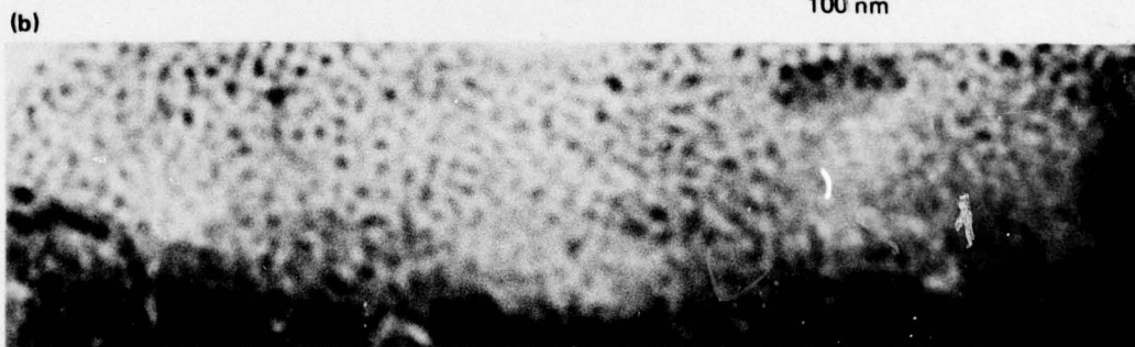
Figure 12 Bright-field transmission electron micrographs of structure in deformed TGDDM-DDS (10 wt% DDS) epoxy
