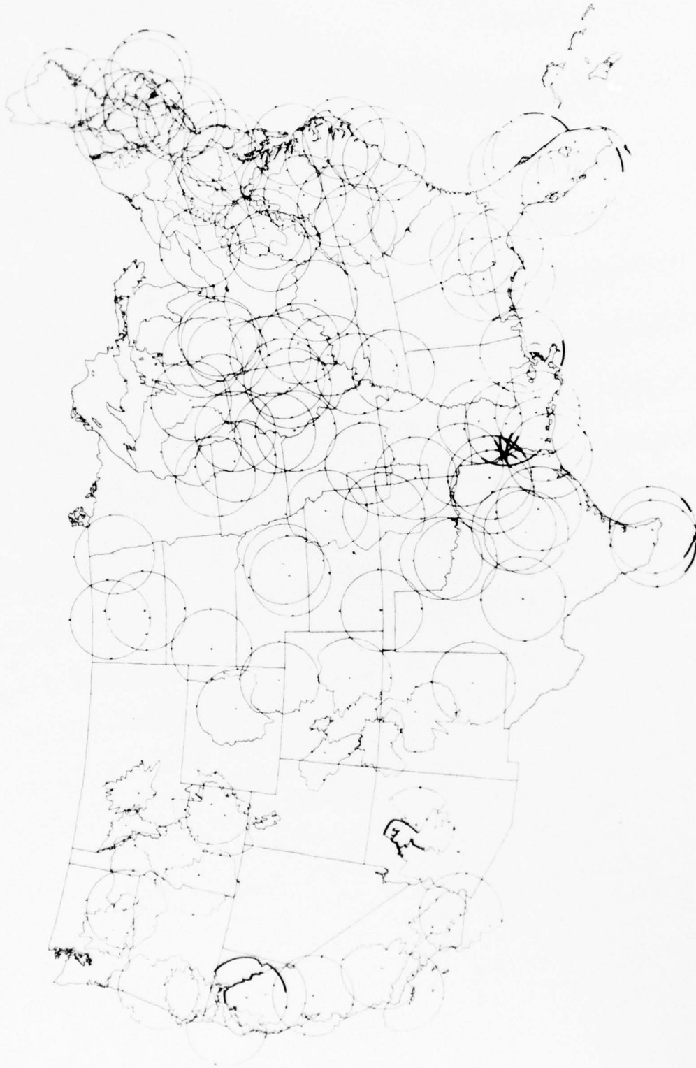
Fig. A.26. Proposed ASR composite coverage map, 15,000 ft. MSL, maximum range R_{\text{max}} = 100 nmi.
