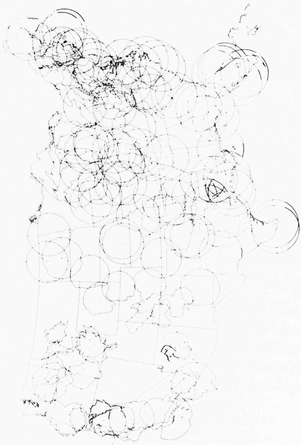
Fig. A.25. Proposed ASR composite coverage map, 15,000 ft. MSL, maximum range R_{\max} \geq 133 nmi.
