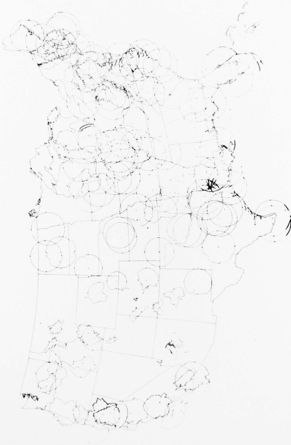
Fig. A.28. Proposed ASR composite coverage map, 10,000 ft. MSL, maximum range R_{max} = 100 nmi.
