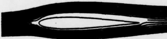
Fig. 12. STREAMLINES AROUND AN IMPULSIVELY STARTED 12X JOUKOWSKI AIRFOIL AT 3^\circ ANGLE OF ATTACK AT EARLY TIME LEVELS
