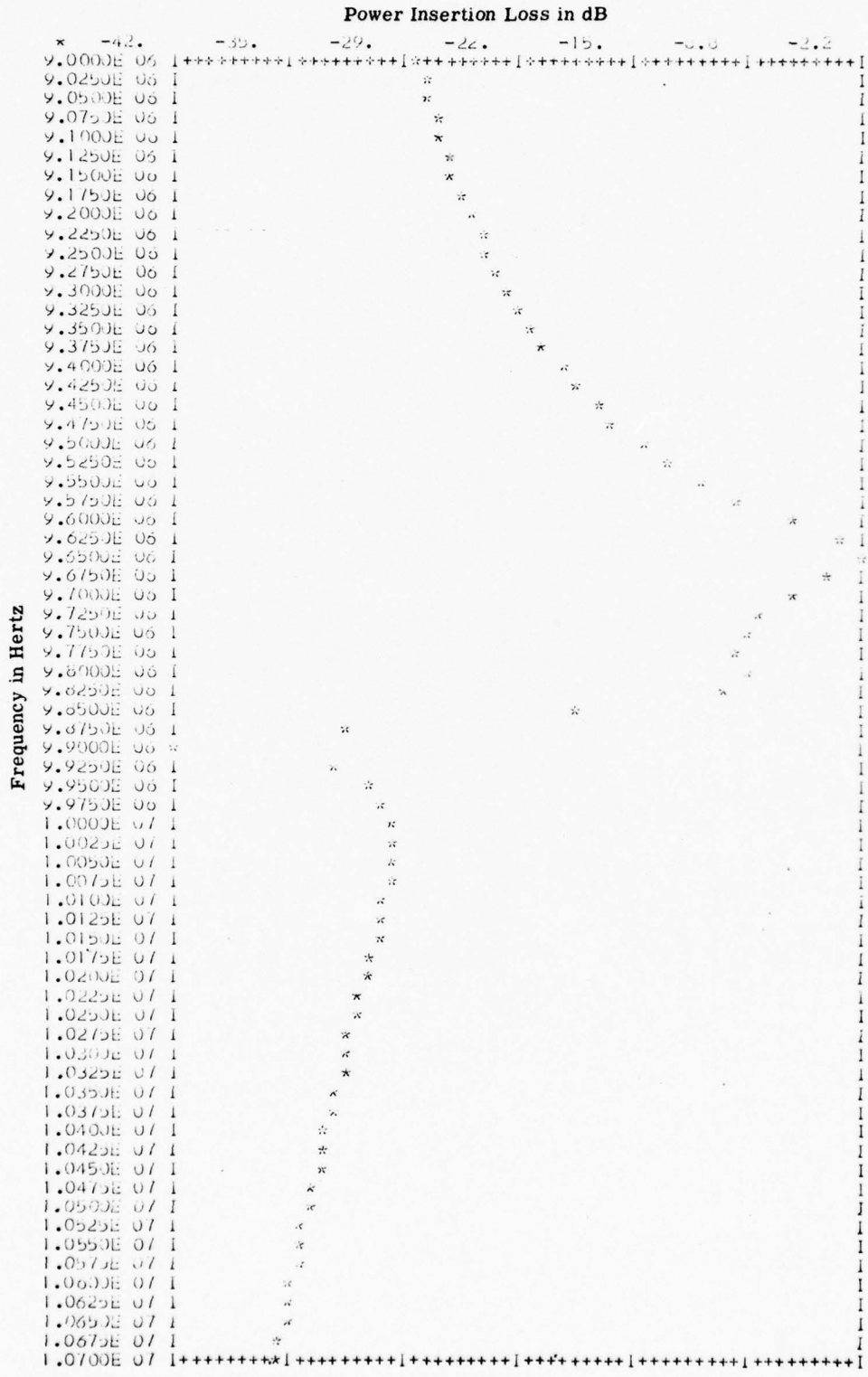
Figure 3-46. Two Element Identical Plate Stack Slower Mode 2 Velocity 70° Rotation Between Plates
