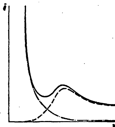
Fig. 58. Character of the dependence of the coefficient of consumption Q on the cavitation number \alpha with a constant Froude number, obtained experimentally. ---- component of gas removal by circular vortices; -.-.- component of gas removal by vortex filaments.
