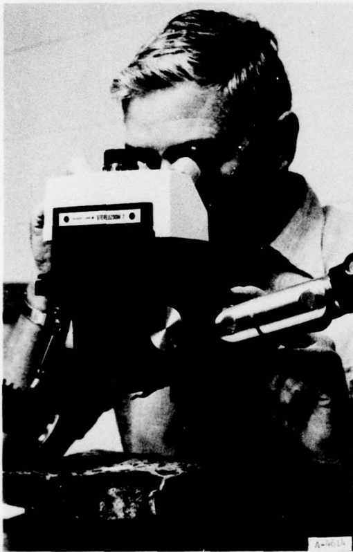
Figure 5. Use of stereoscopic microscope to examine concrete
