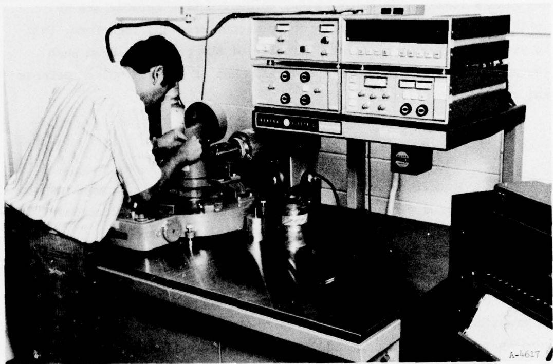
Figure 6. X-ray diffractometer for the examination and identification of crystalline materials
