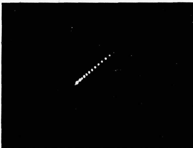
Figure 4.16a Showing the Output of a 13 Mode Polyurethane TWG when TE_0 was Excited on the Primary WG.
