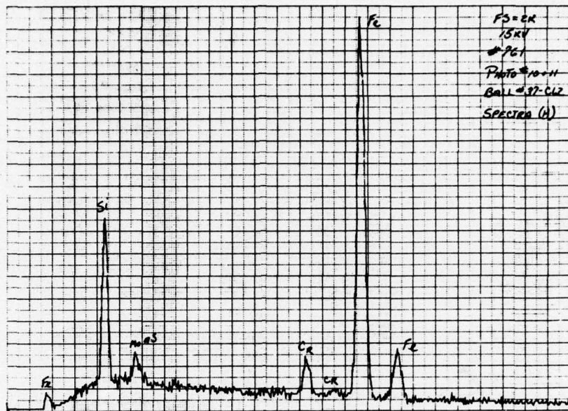
Figure 51 Electron Microprobe Trace P/M M-50 Ball S/N 37. This trace revealed the presence of silicon. This ball spalled after 108.7 million stress cycles.
