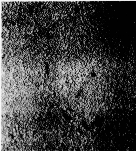
Figure 13 Powder Metal Processed EX00007 Alloy. The M-50/T-15 powder metal processed alloys were free of non-metallic contamination as was the powder metal processed EX00007 alloy.
