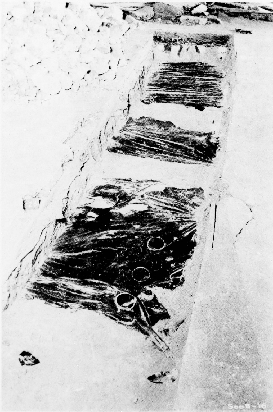
Figure 51. Polyethylene Membrane on Bottom of MESL After Traffic, Item 2
