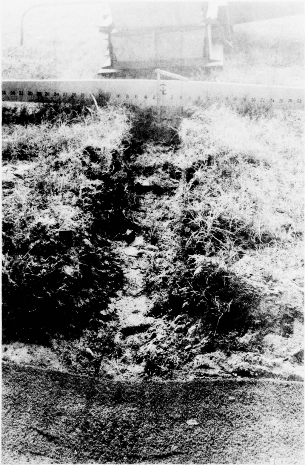
Figure 48. Rut in Item 5 After One Pass
