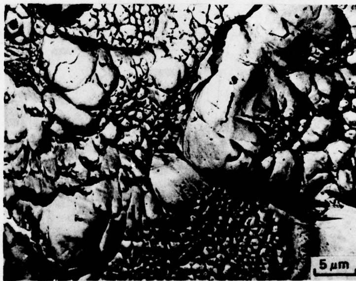
Fig. 5. Fractograph (EM) of overload fracture in dry air showing dimples on an intercrystalline facet.
