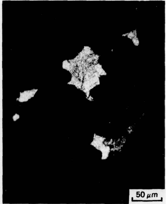
Fig.13. Fractograph (optical) after sub-critical crack growth induced by liquid alloy showing that most of the fracture surface is covered by a thin film of alloy and that small areas (light regions) had fractured without being 'wet' with liquid alloy.
