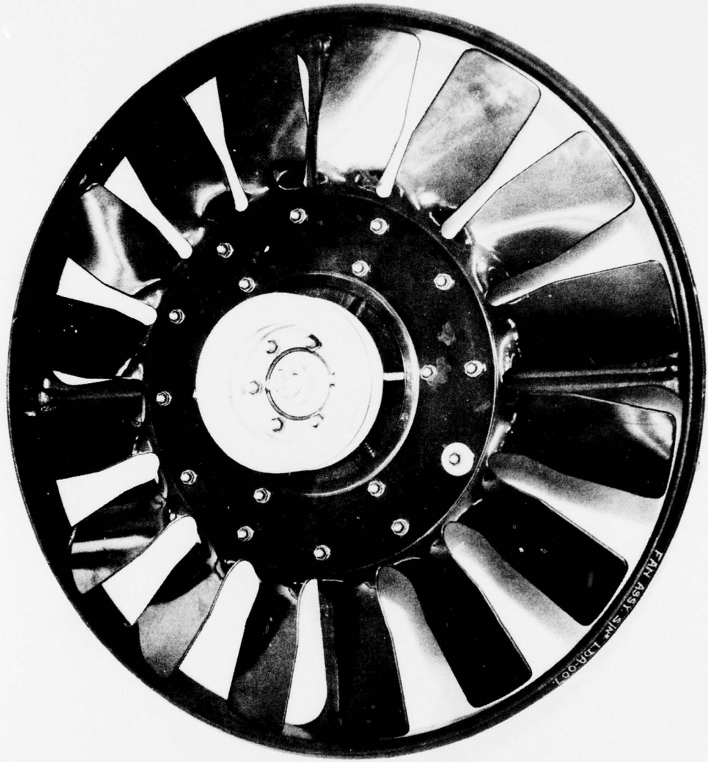
FIG. 1. THE COOLING FAN ASSEMBLY - FRONT FACE
