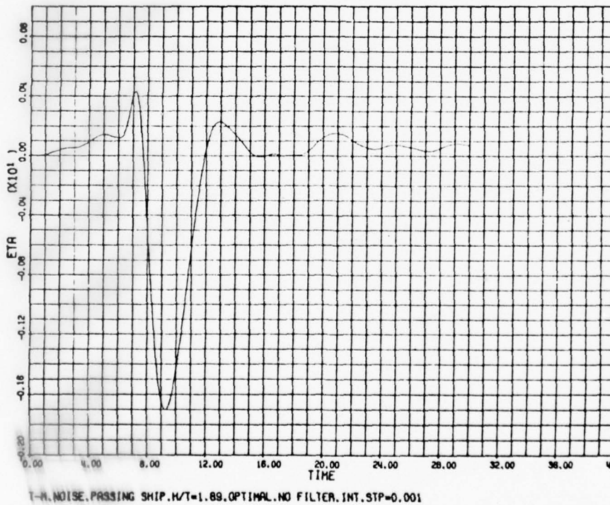
Figure 17. Lateral Offset Response to Passing Ship: Optimal Design without Shaping Filters
