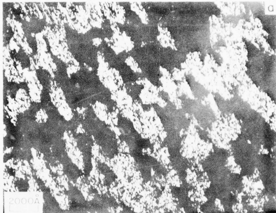
Fig. 71 TEM of GaAs implanted with 400 keV Se ions and annealed at 200°C for 1100 minutes. (a) Dark field image illustrating crystalline substructure in implanted layer. g: \langle 111 \rangle streak. (b) Selected area diffraction pattern, [110] zone normal with intense \langle 111 \rangle streaking.
