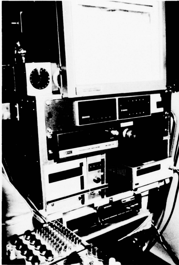
FIG. 6: CLOSE-UP VIEW OF IN-VEHICLE TEST INSTRUMENT READ-OUTS
