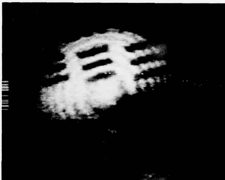
Figure 12. Air Force resolution target viewed through TIFIS system. Total field of view is 5 mrad. Target bars at upper half of picture are 0.5 mrad center to center.
