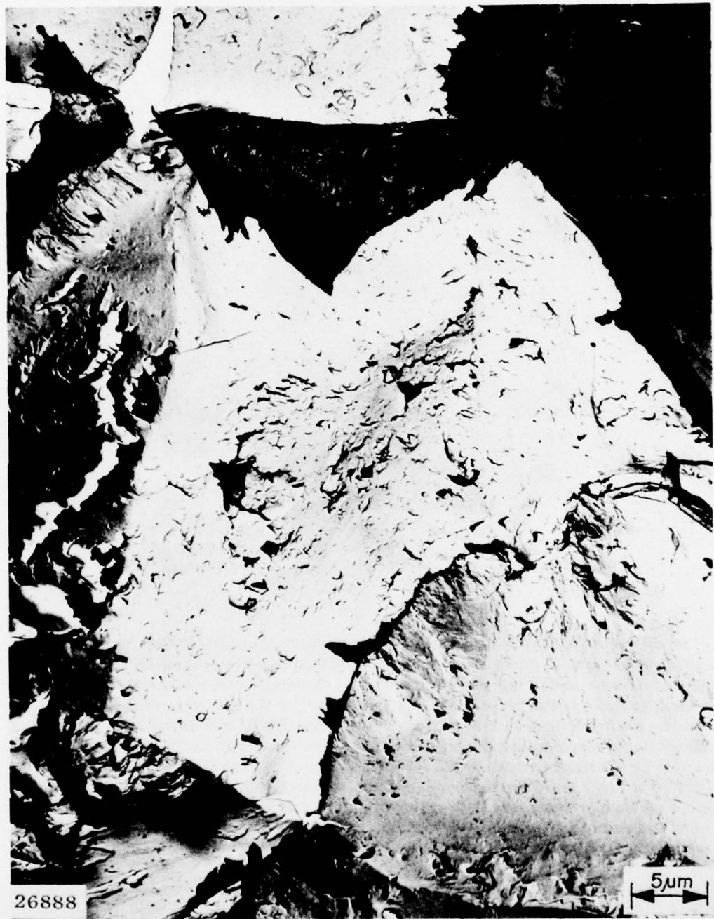
Fig. 54 — TEM fractograph showing intergranular fracture in hydrogen flake detected in LB weld of 12.7-mm-thick HY-130 DT specimen
