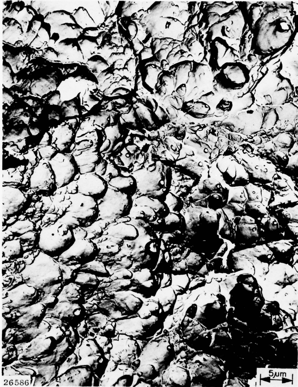
Fig. 42 — Microvoid coalescence in weld metal in midthickness region of GMA weld joint fracture of 12.7-mm-thick HY-130 DT specimen.
