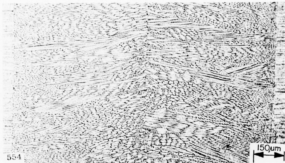
Fig. 33 — Solidification structure of weld metal at midthickness of 6.35-mm-thick HY-130 EB weldment preheated \sim 120^{\circ}\text{C} . Etched in 0.5% ammonium persulphate.
