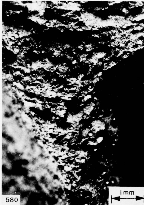
Fig. 44 — Pop-in region in weld metal of EB weld joint fracture of 12.7-mm-thick HY-130 DT specimen. Preheated \sim 120^{\circ}\text{C} . Note gas pockets in fracture.
