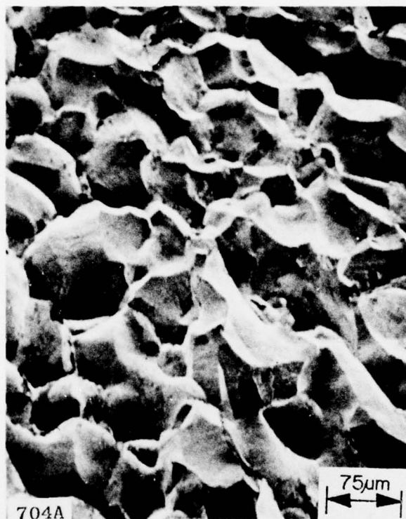
Fig. 55 — SEM fractograph showing intergranular fracture in hydrogen flake detected in LB weld of 12.7-mm-thick HY-130 DT specimen
