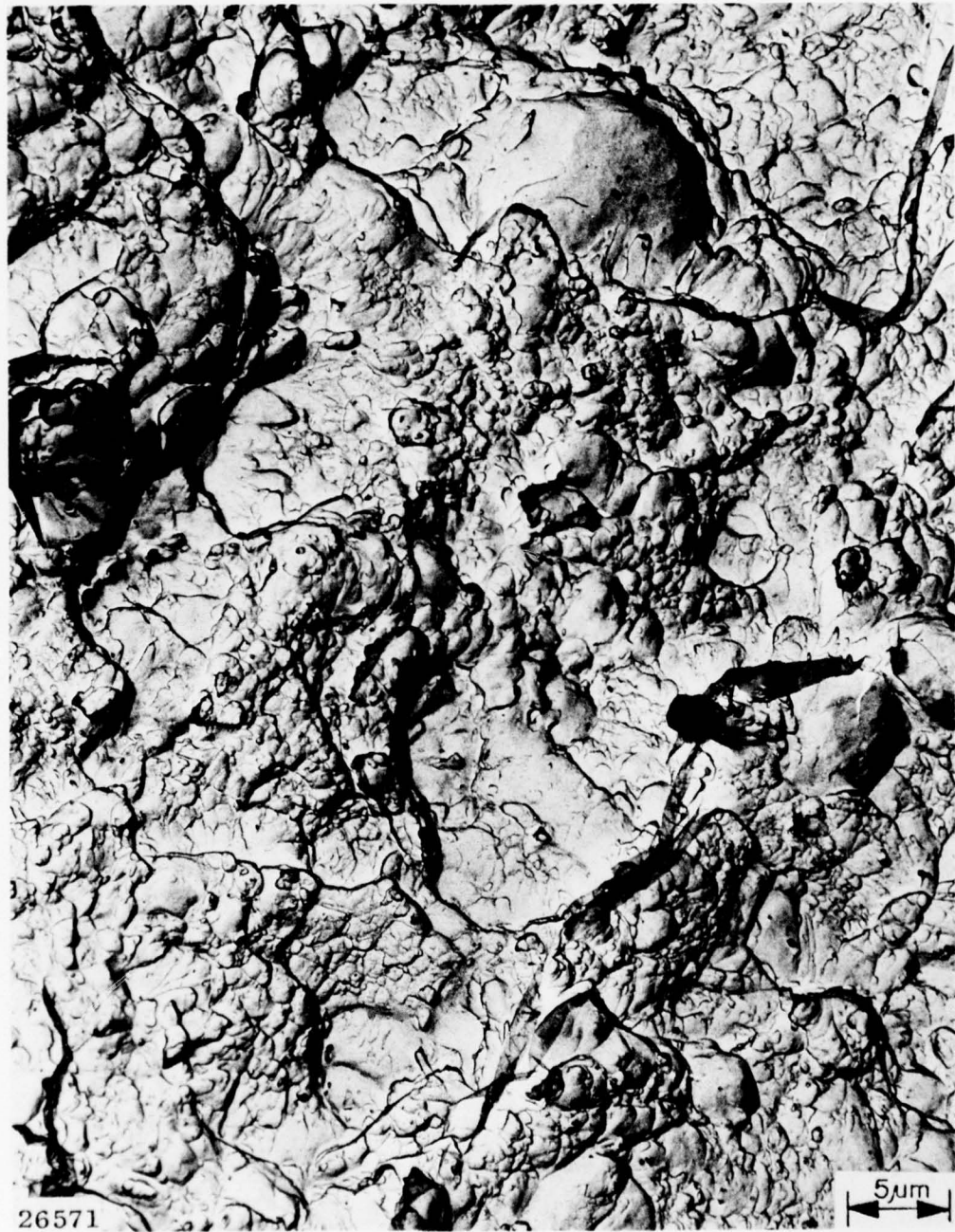
Fig. 47 — Microvoid coalescence in unaffected base metal in EB weld joint fracture of 12.7-mm-thick HY-130 DT specimen. Not preheated.
