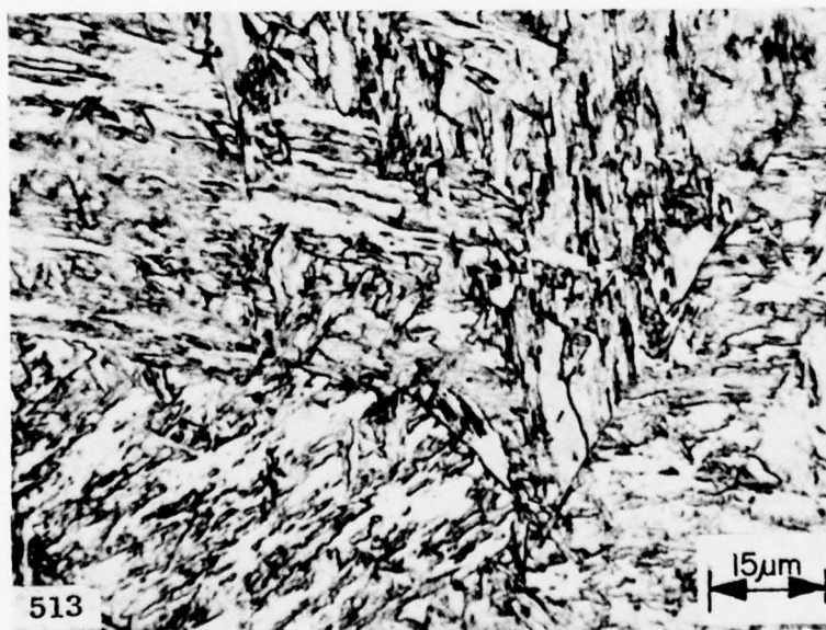
Fig. 8 — Acicular ferrite, martensite, and bainite in weld metal of 6.35-mm-thick GMA weldment. Hardness 37.5 Rc. Etched in 1% nital.
