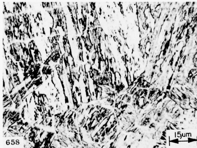
Fig. 22 — Martensite and bainite in weld metal of 12.7-mm-thick HY-130 LB weldment. Hardness 38.5 Rc. Etched in 1% nital.
