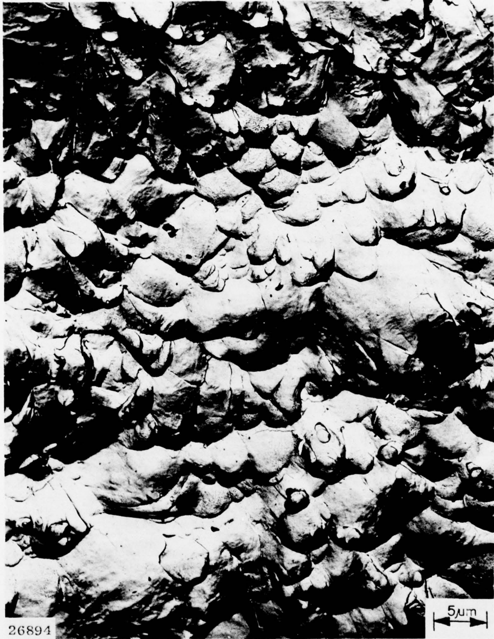
Fig. 56 — Microvoid coalescence in highly fissured region below hydrogen flake in LB weld of 12.7-mm-thick HY-130 DT specimen
