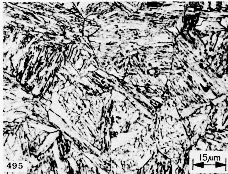
Fig. 11 — Bainite in coarse grain region of HAZ adjacent to fusion boundary in 6.35-mm-thick HY-130 SMA weldment. Hardness 36.5 Rc. Etched in 1% nital.
