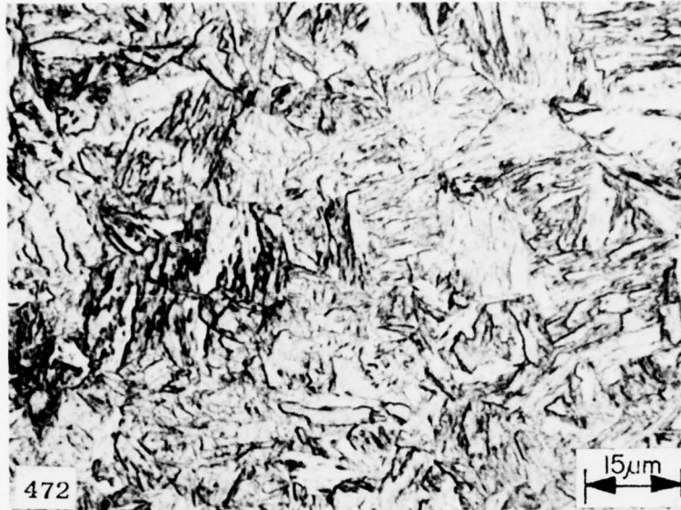
Fig. 27 — Martensite and some bainite in medium grain region of HAZ adjacent to fusion boundary in 12.7-mm-thick HY-130 EB weldment. Hardness 38.0 Rc. Etched in 1% nital.
