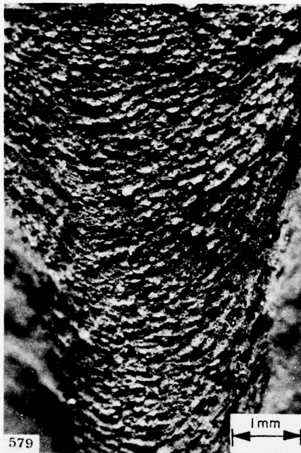
Fig. 40 — Pop-in region in weld metal of GMA weld joint fracture of 12.7-mm-thick HY-130 DT specimen.
