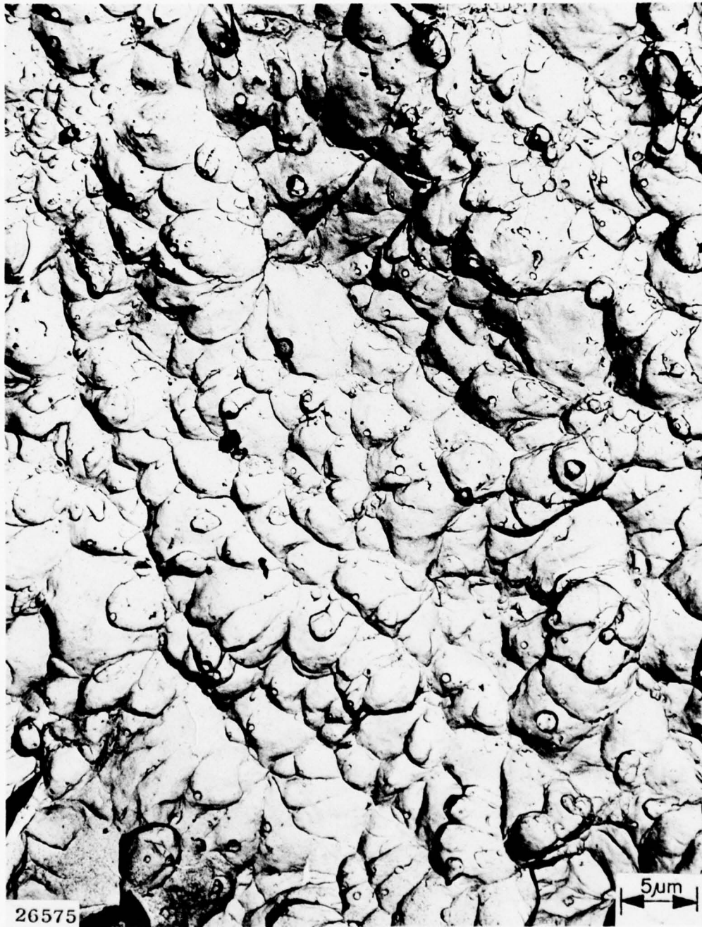
Fig. 41 — Microvoid coalescence in pop-in region in weld metal of GMA weld joint fracture of 12.7-mm-thick HY-130 DT specimen.
