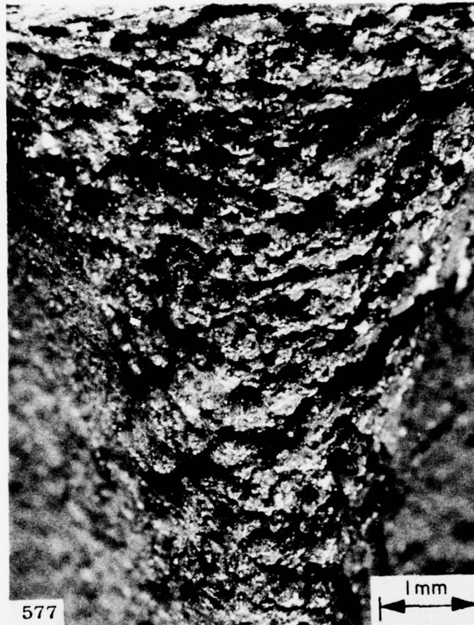
Fig. 48 — Pop-in region of fracture in 12.7-mm-thick base metal DT specimen.
