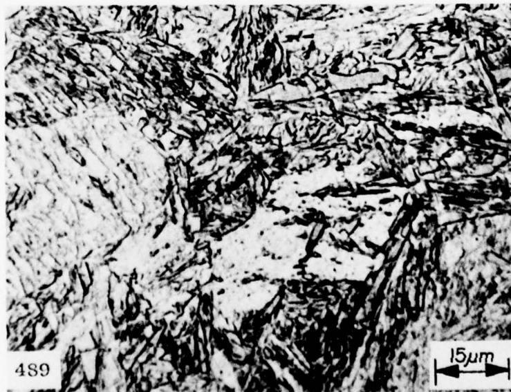
Fig. 10 — Martensite and some bainite in weld metal of 6.35-mm-thick LB weldment. Hardness 42.0 Rc. Etched in 1% nital.
