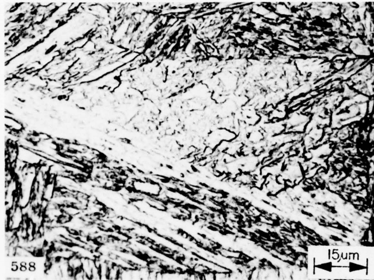
Fig. 21 — Martensite and bainite in weld metal of 12.7-mm-thick HY-130 EB weldment. Hardness 37.5 Rc. Etched in 1% nital.
