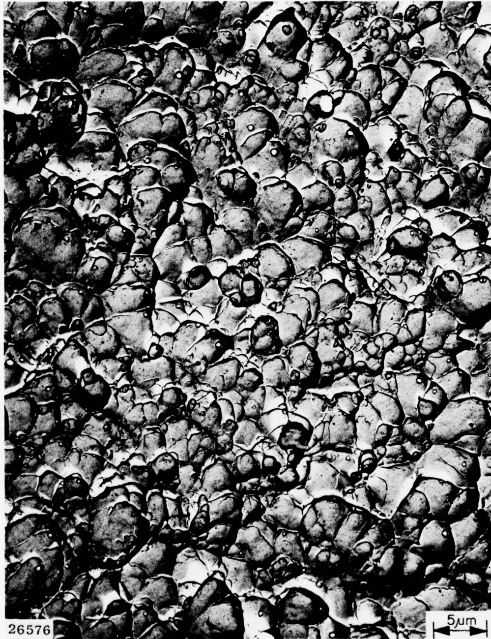
Fig. 43 — Microvoid coalescence in weld metal near surface of GMA weld joint fracture of 12.7-mm-thick HY-130 DT specimen.
