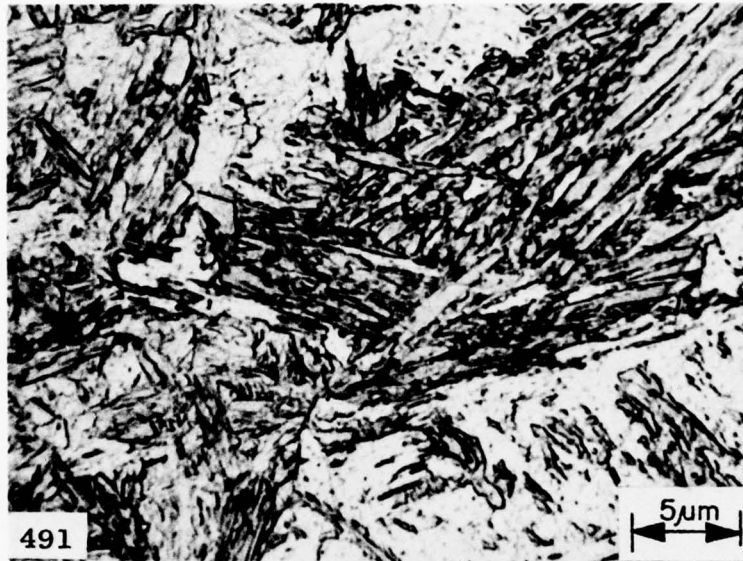
Fig. 17 — Martensite and some bainite in medium grain region of HAZ adjacent to fusion boundary in 6.35-mm-thick HY-130 LB weldment. Hardness 40.5 Rc. Etched in 1% nital.
