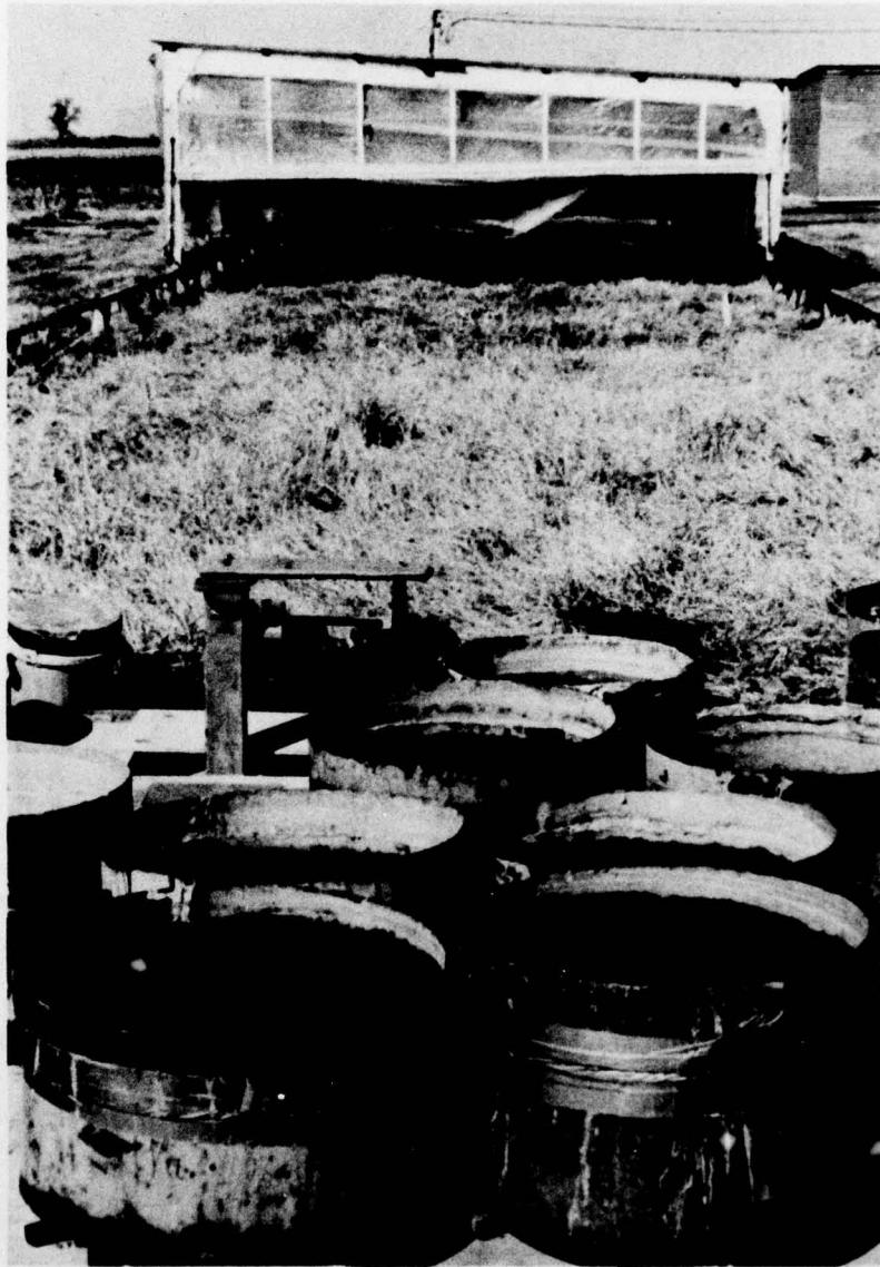
Figure 32. General view of the field location showing the containers of dredged material, the scale, and the rain shelter in the off position
