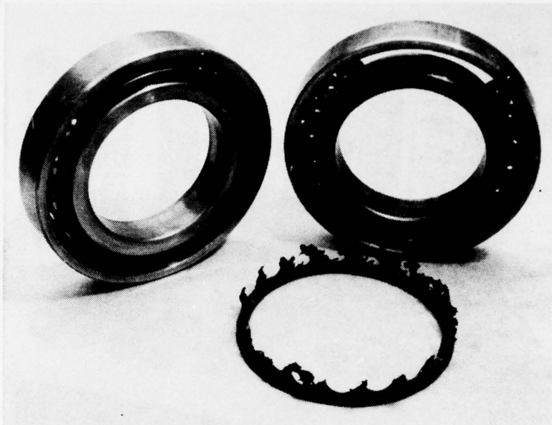
Figure 81. Fan accessory drive duplex bearing showing melted nylatron retainer after 19-minute loss-of-lube test of transmission number 2.
