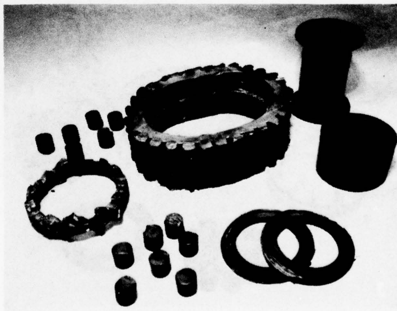
Figure 99. Lower planetary pinion, bearing, inner race, rollers, retainer, and roller guides after fourth loss-of-lube test.
