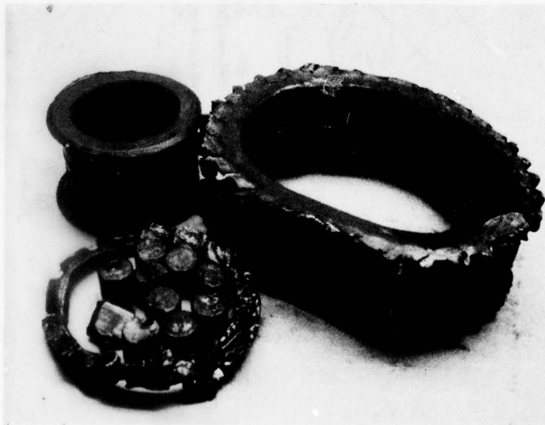
Figure 36. Lower planetary pinion, bearing inner race, rollers, roller guides, and retainer after 21-minute loss-of-lube retest of transmission number 1.
