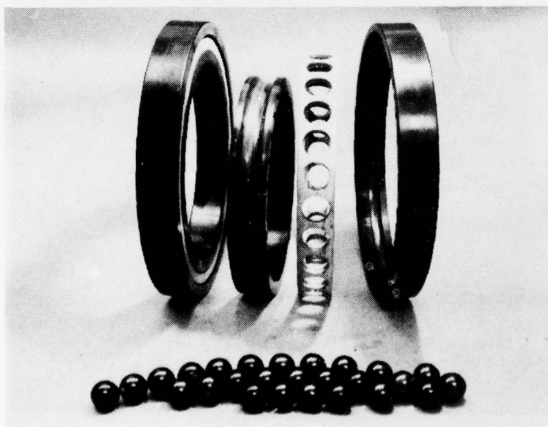
Figure 80. Main gearshaft duplex bearing after 19-minute loss-of-lube test of transmission number 2.
