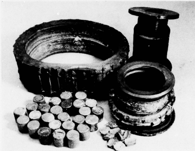
Figure 69. Oblong lower planetary pinion, bearing inner race, rollers, retainer, and roller guides after 19-minute loss-of-lube test of transmission number 2.
