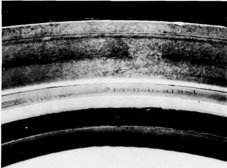
Figure 112. Main input carbon radial seal after fourth loss-of-lube test.
