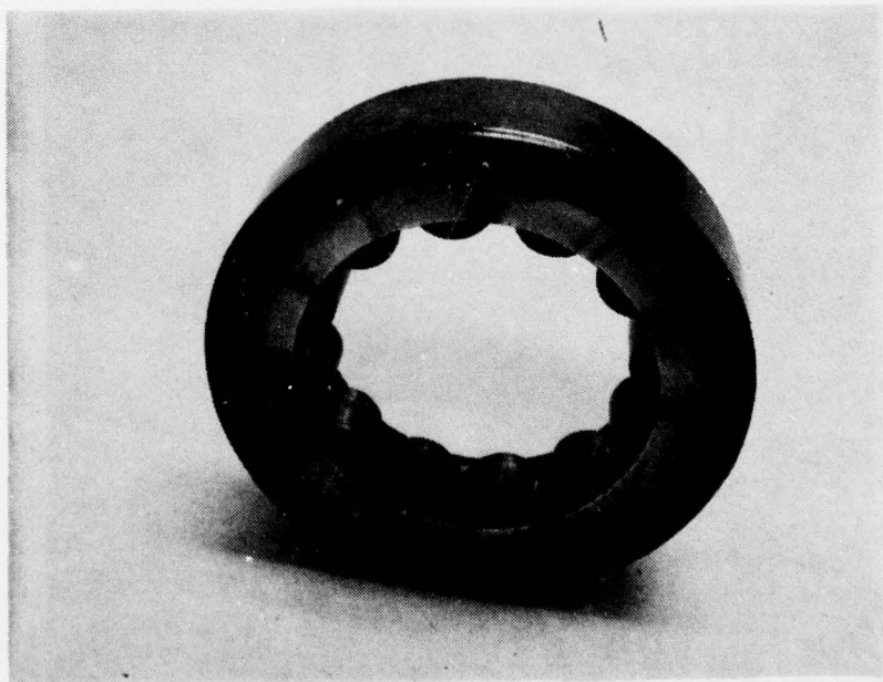
Figure 111. Input pinion roller bearing following fourth loss-of-lube test.
