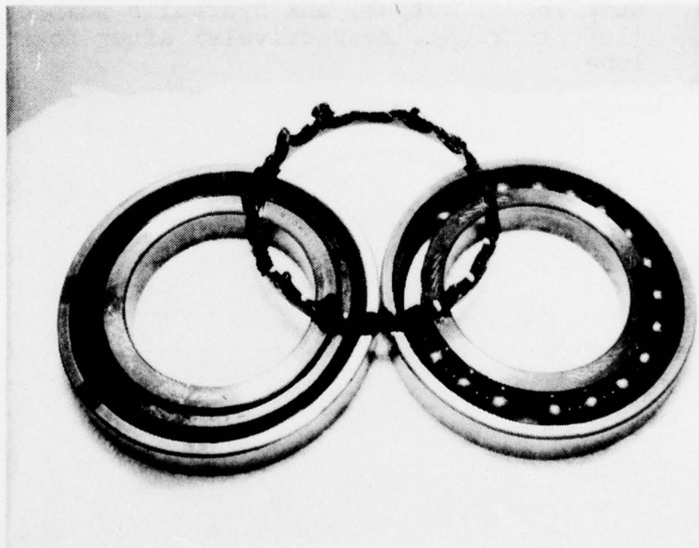
Figure 115. Fan accessory drive duplex bearing after fourth loss-of-lube test.
