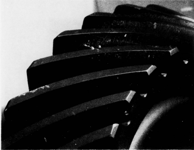
Figure 77. Main input pinion teeth (drive side) showing moderate scoring after 19-minute loss-of-lube test of transmission number 2.
