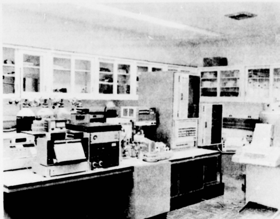
Figure 3. Gas chromatograph-mass spectrometer-data system used for analysis.
