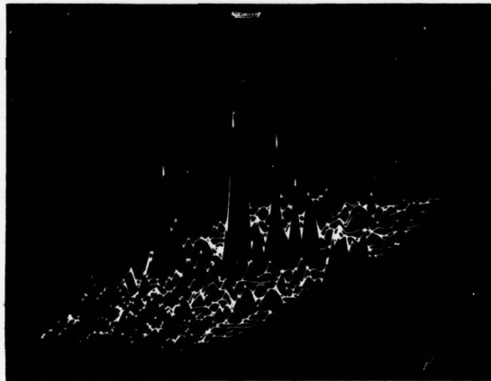
(c) Highway correlogram Image SNR = 10 db Correlation SNR = 18.6 db
