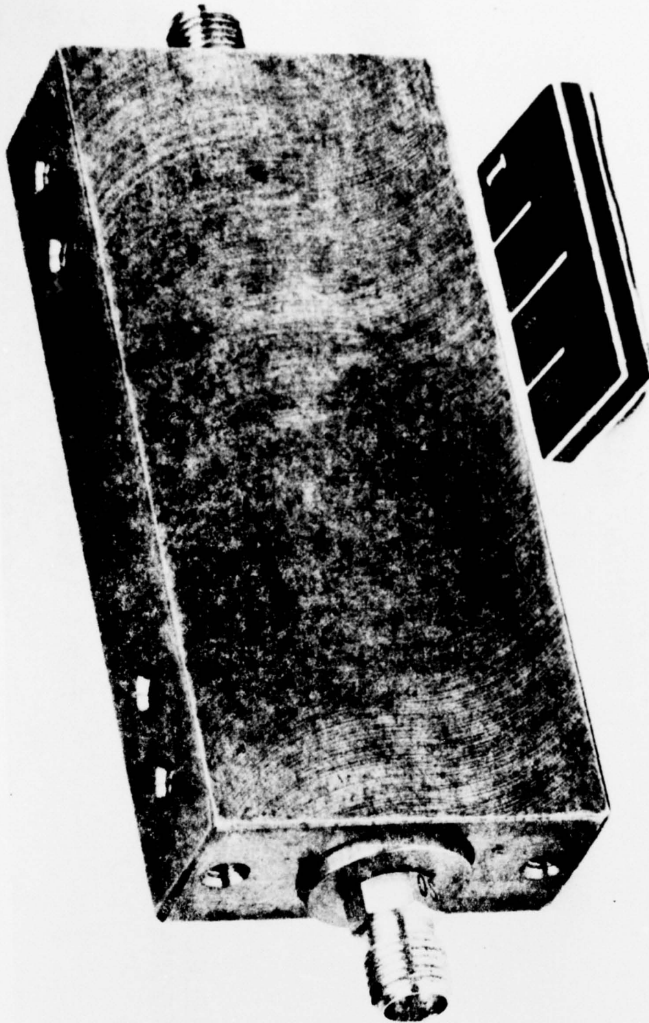
FIGURE 5 - EXTERNAL VIEW OF YIG-ROD FERRITE LIMITER
