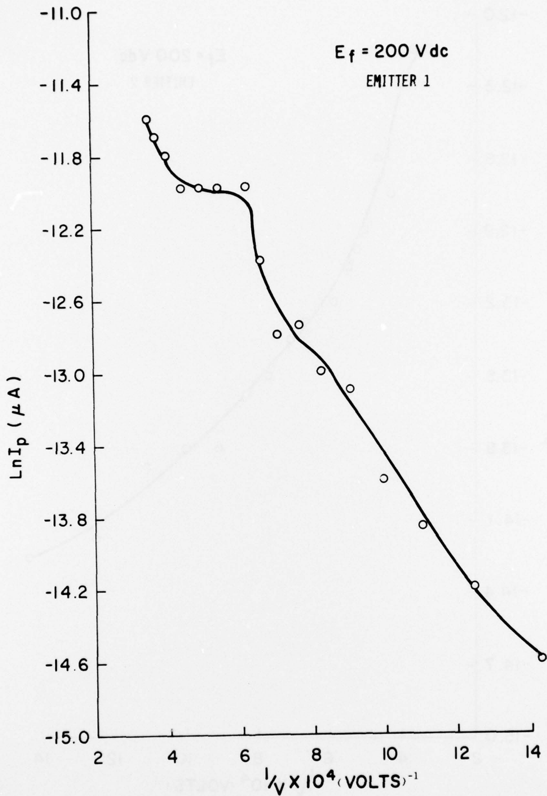
FIG. 15 MODIFIED FIELD PLOT OF \text{SnO}_2 COLD CATHODE (EMITTER 1)
