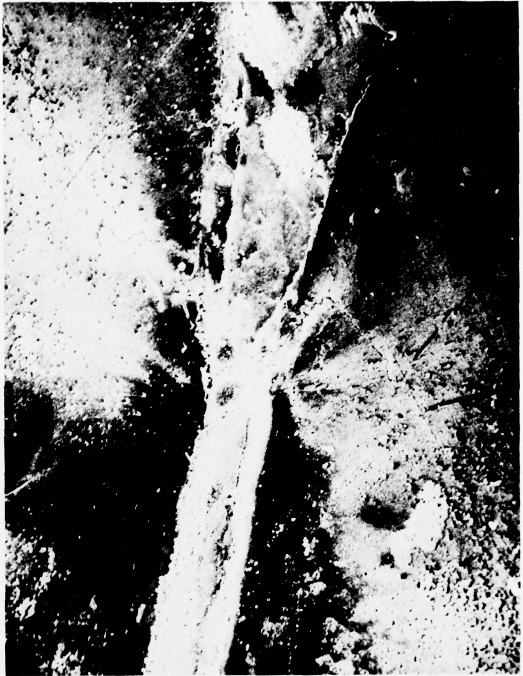
FIG 10a ELECTRON MICROGRAPH OF EMITTING REGION OF SINGLE ELEMENT \text{SnO}_2 EMITTER.
