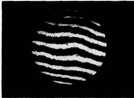
Figure 25. Interferogram of a Holographic Optical Element When Used as a Collimating Lens.
