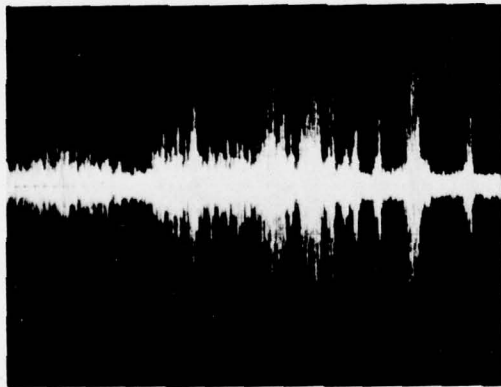
(c) FORT SILL GROUP FIRING IMPACT (76 PIECES) HORIZONTAL 1 s/cm +G = 0.2 10-s DURATION
