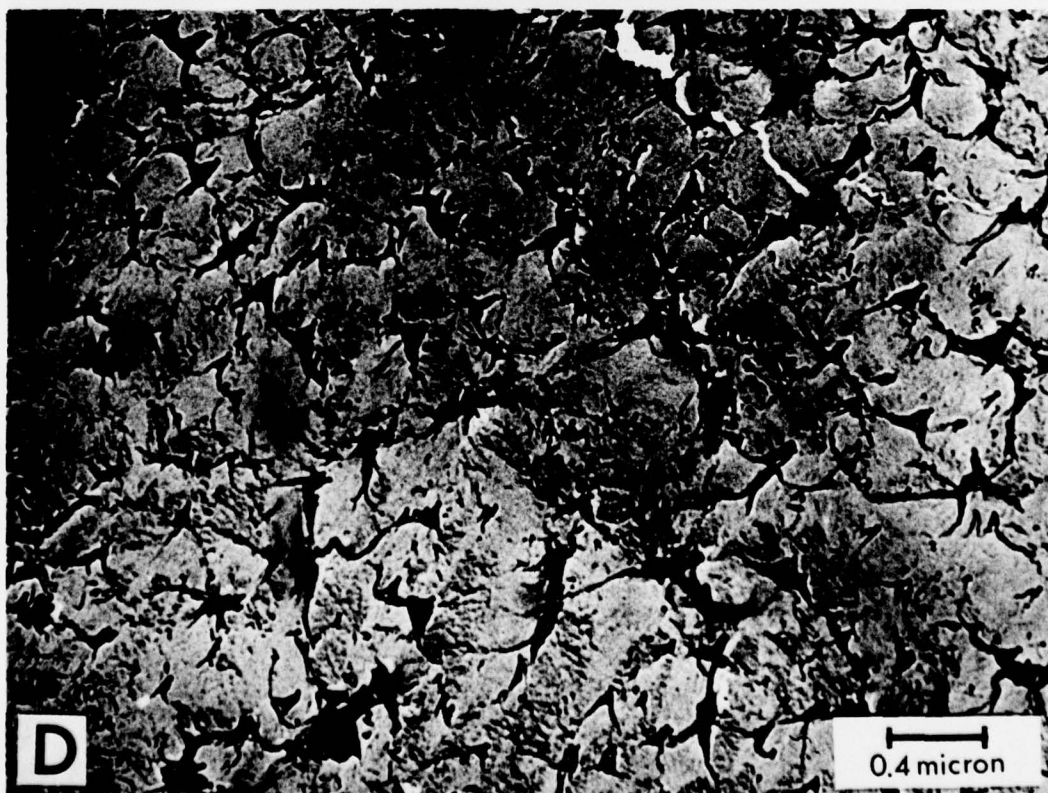
Figure 2. Replicate TEM micrographs showing progressive phase separation and crystallization in the 000 glasses. (C) 290°C - 6 hrs. and (D) 410°C - 6 hrs. (bar = 0.5 \mu m).
