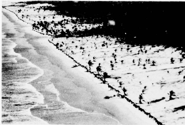
Figure 35. Photograph of the beach in the vicinity of the Plantation site showing the transgressive dune field and the erosion scarp undermining the coconut trees.
