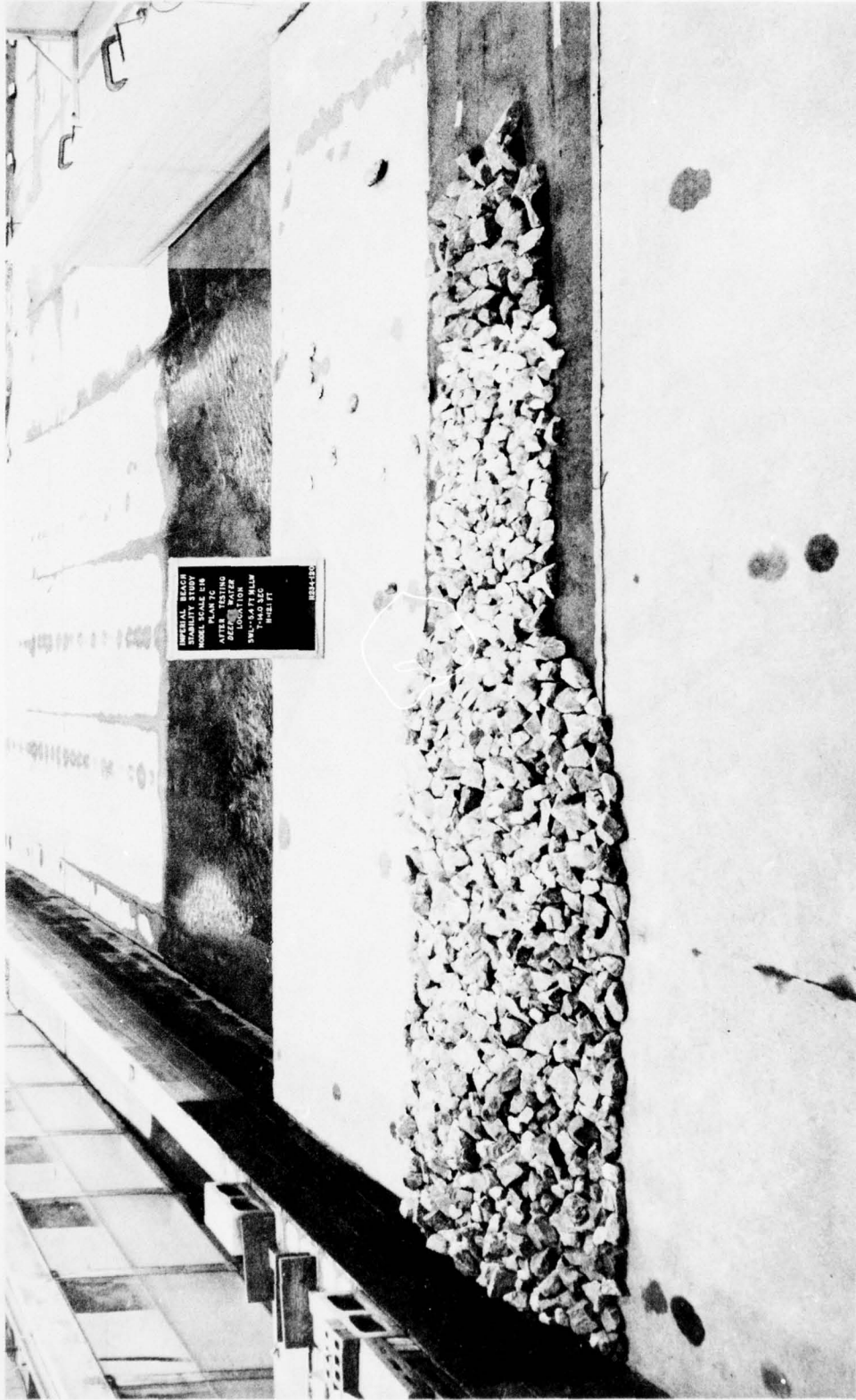
Photo 38. Sea-side view of Plan 7C in the deeper water location after 4.0 hr of 14.0-sec, 12.1-ft waves at an swl of +5.4 ft mllw
