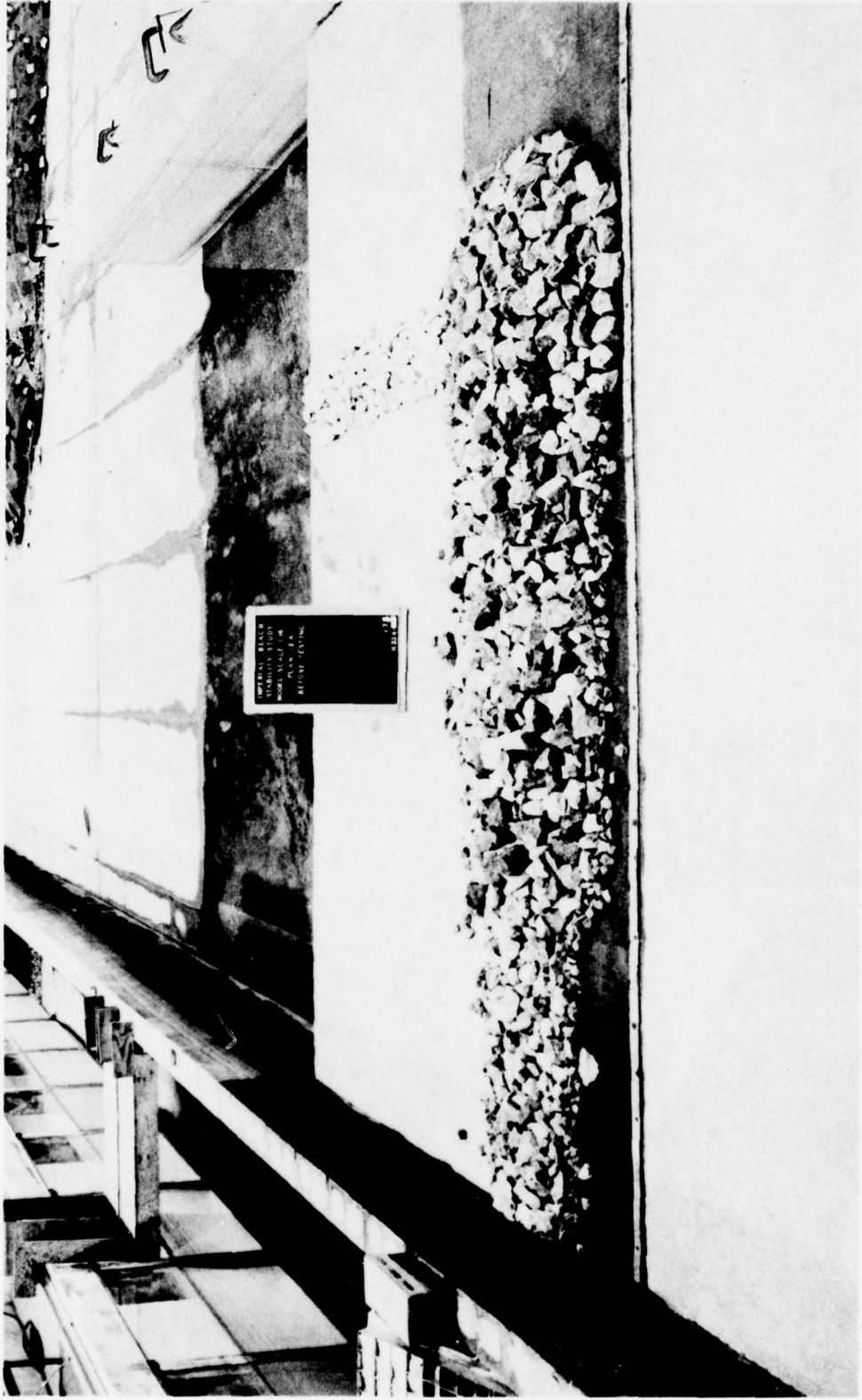
Photo 66. Sea-side view of Plan 12A before wave attack
