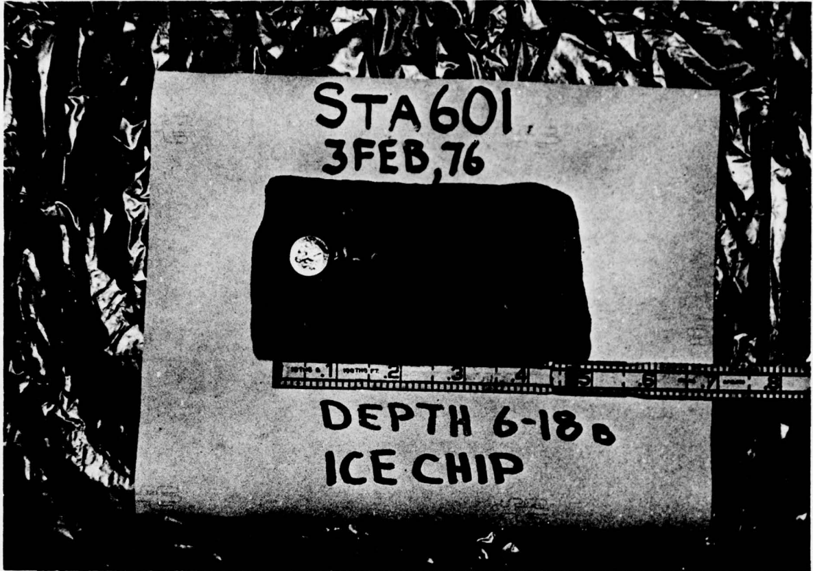
23. Alger County. State Road 28. Close-up of core showing ice chip incorporated into compacted soil.
