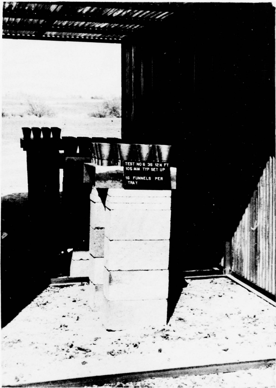
Fig 4 Typical arrangement - test without shields.
