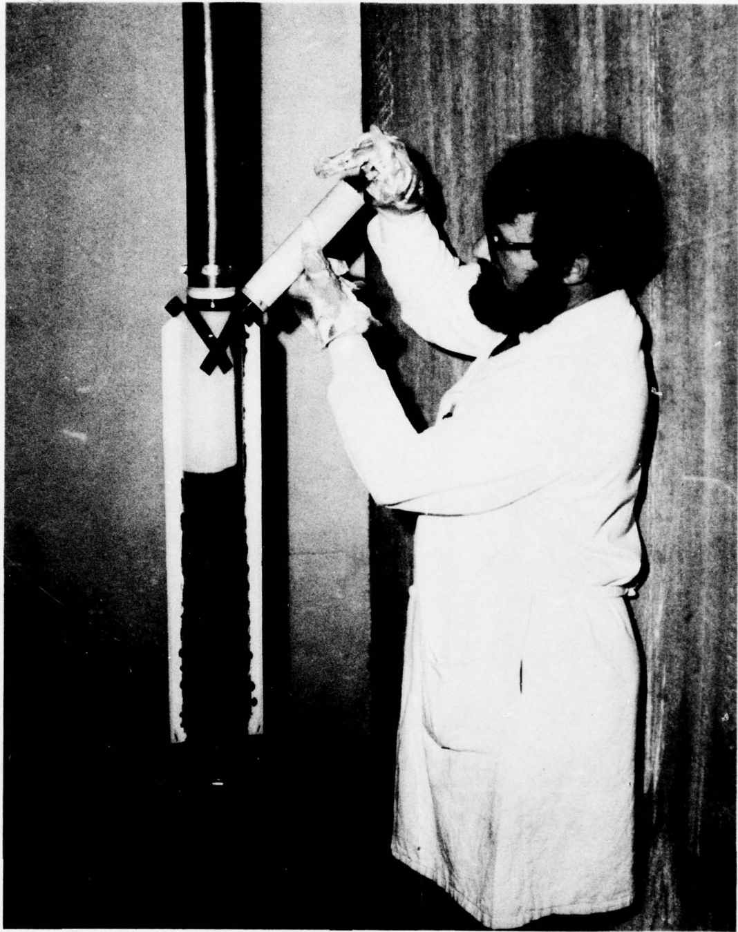
Figure 24. Injection of polyurethane mixture into mold.
