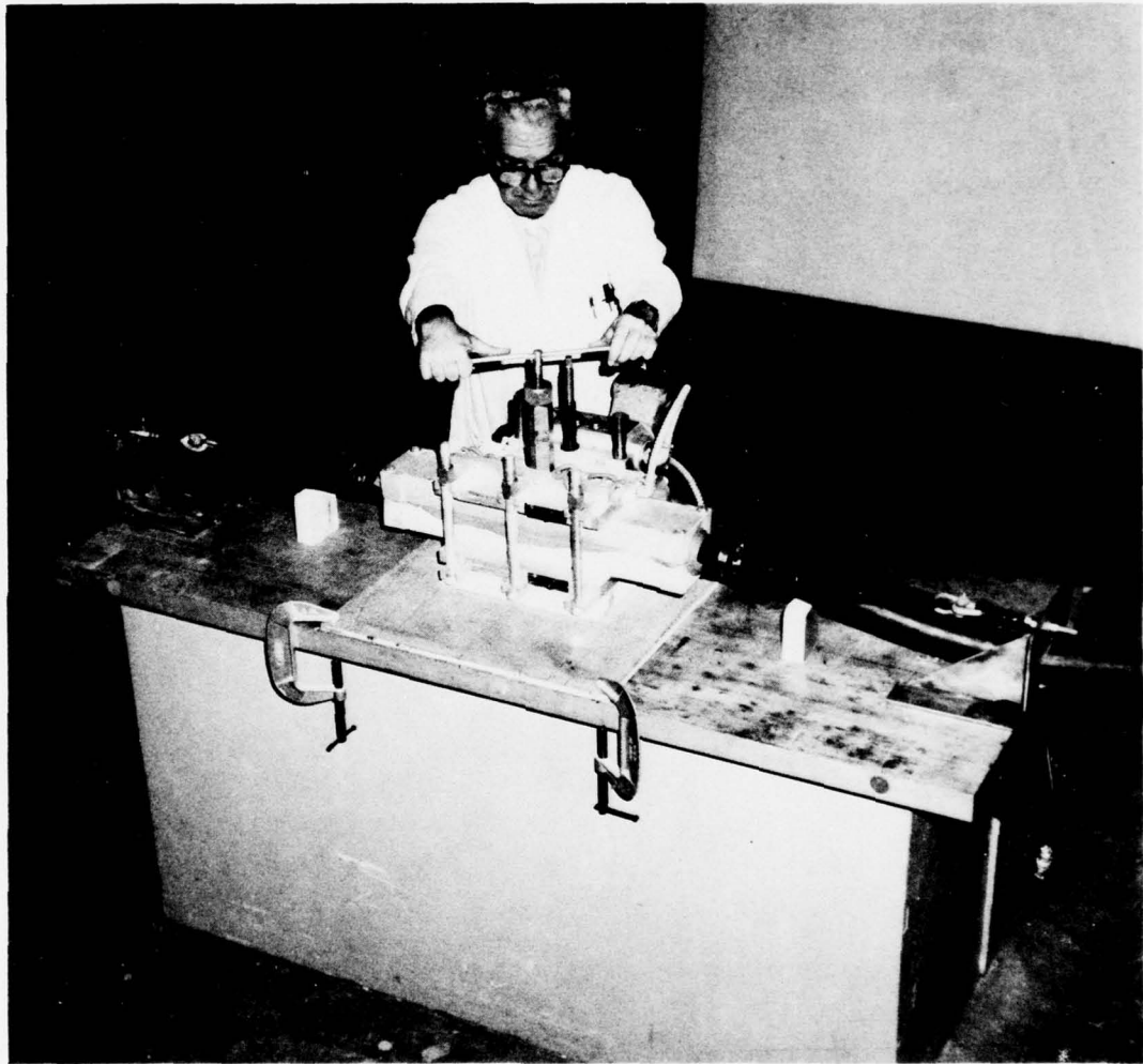
Figure 19. Injection of neoprene from transfer pot.
