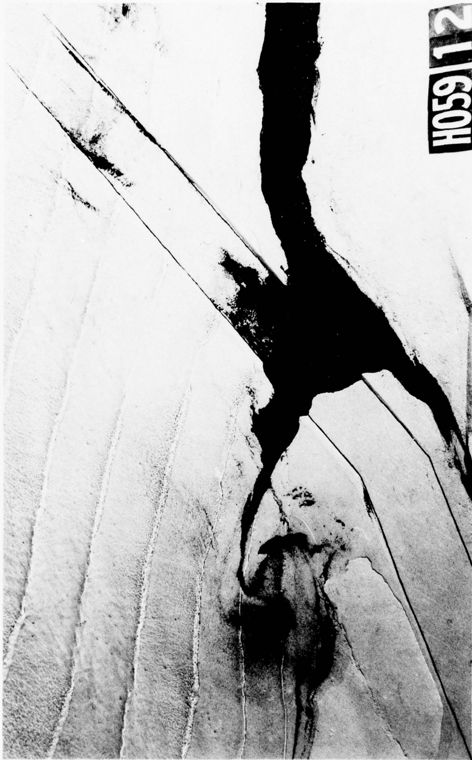
Photo 12. Typical wave and shoaling patterns for Plan 1; 7.3-sec, 8.3-ft waves from 330°, 1,500-cfs discharge, swl = +2.0 ft lwd
