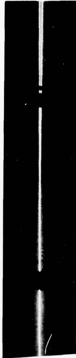
Figure 6: Observed break-up of a parent linearly polarized beam, incident on the Na vapor from the left, into two coherent daughter beams of opposite circular polarization, equal intensity, and symmetrical deviation from the parent direction. The splitting angle increases as cell temperature and sodium density increases.
