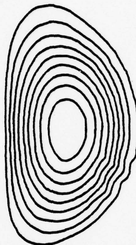
Fig. 7 Vorticity Contours, Reynolds Number = 250 60 time steps, Modified Program.
