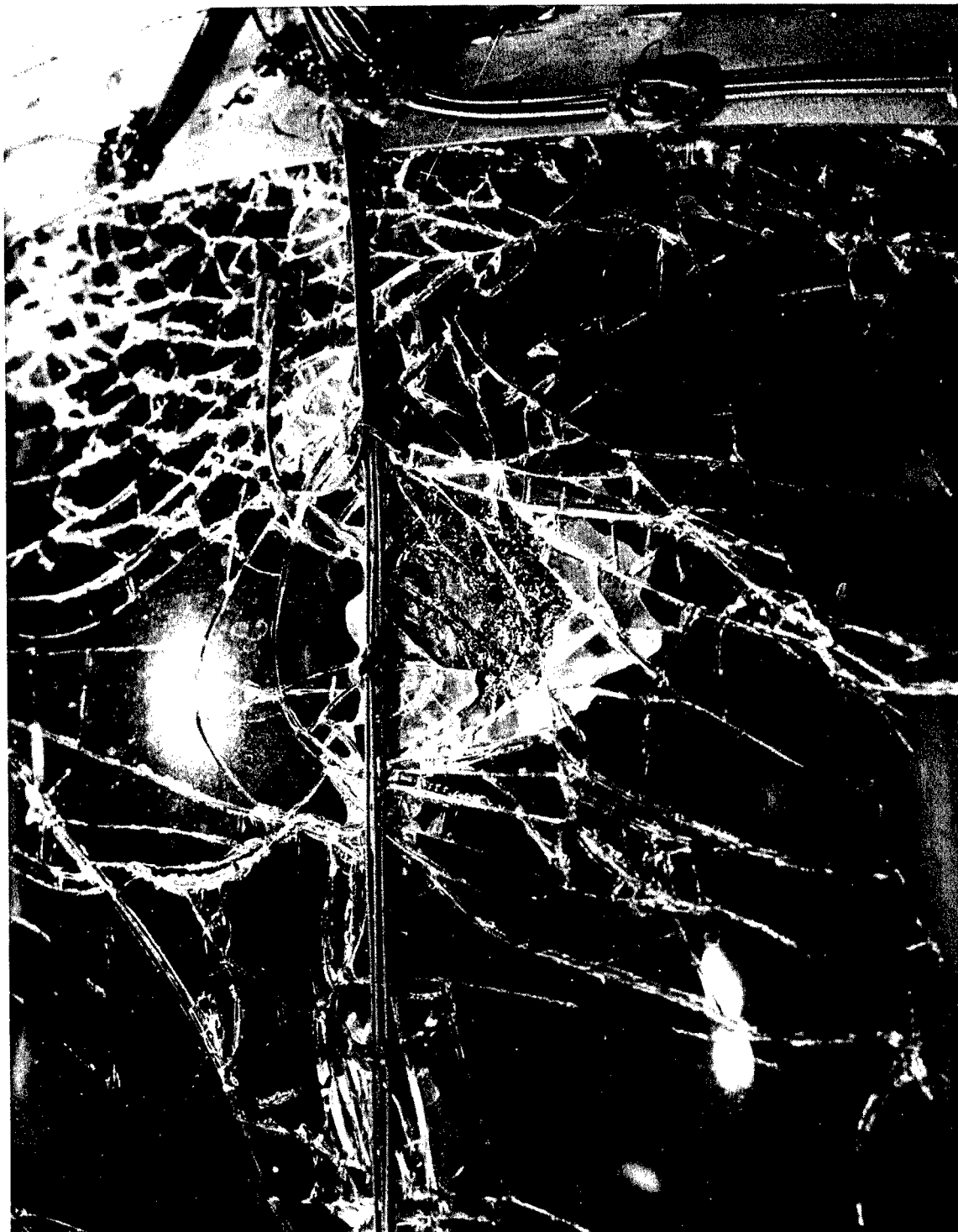
Figure 22. Exposed Cast-In-Place Interlayer of the Left Canopy at the End of Three Lifetimes of Testing
