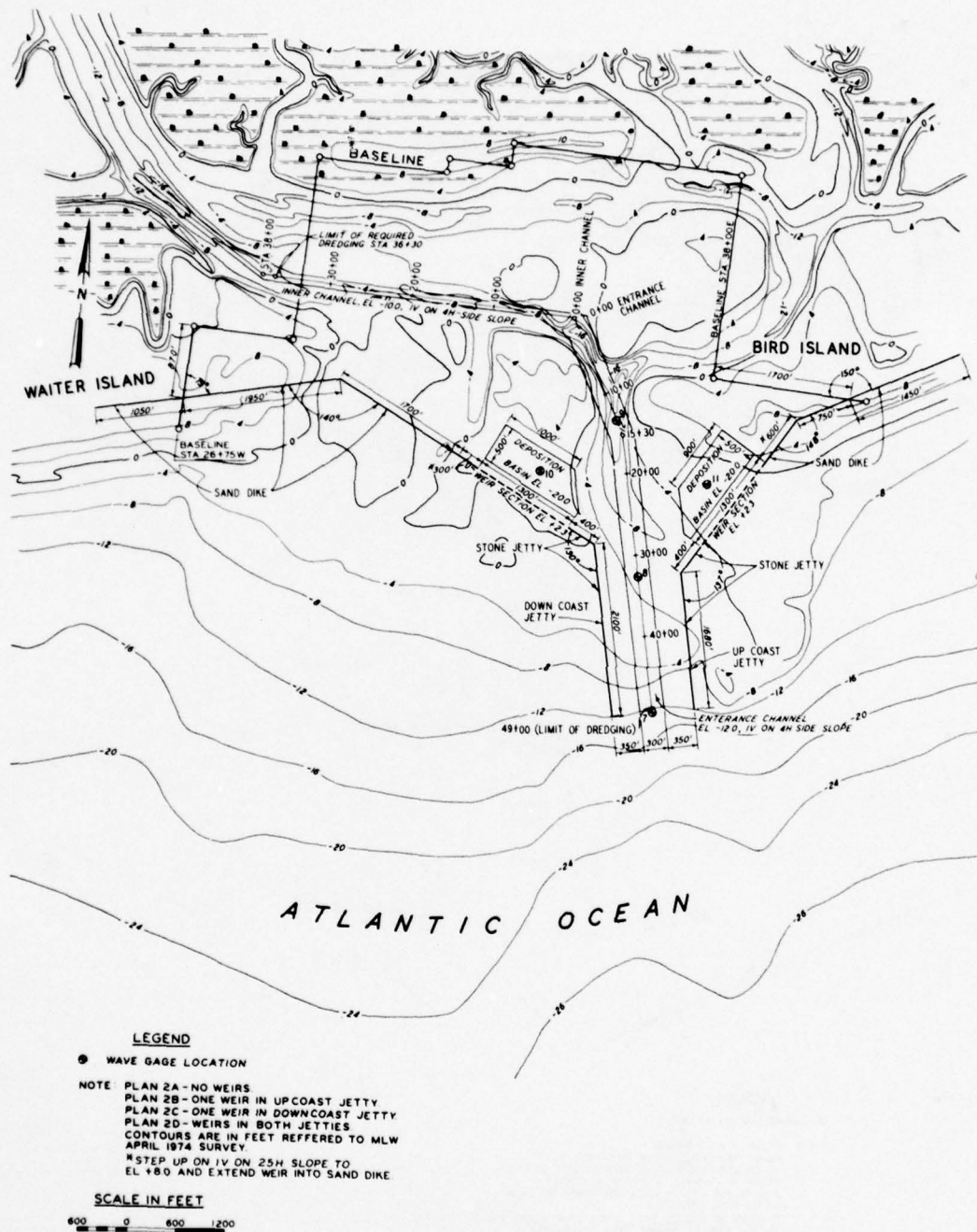
Figure 28. Jetty and channel alignment for Plans 2A, 2B, 2C, and 2D
