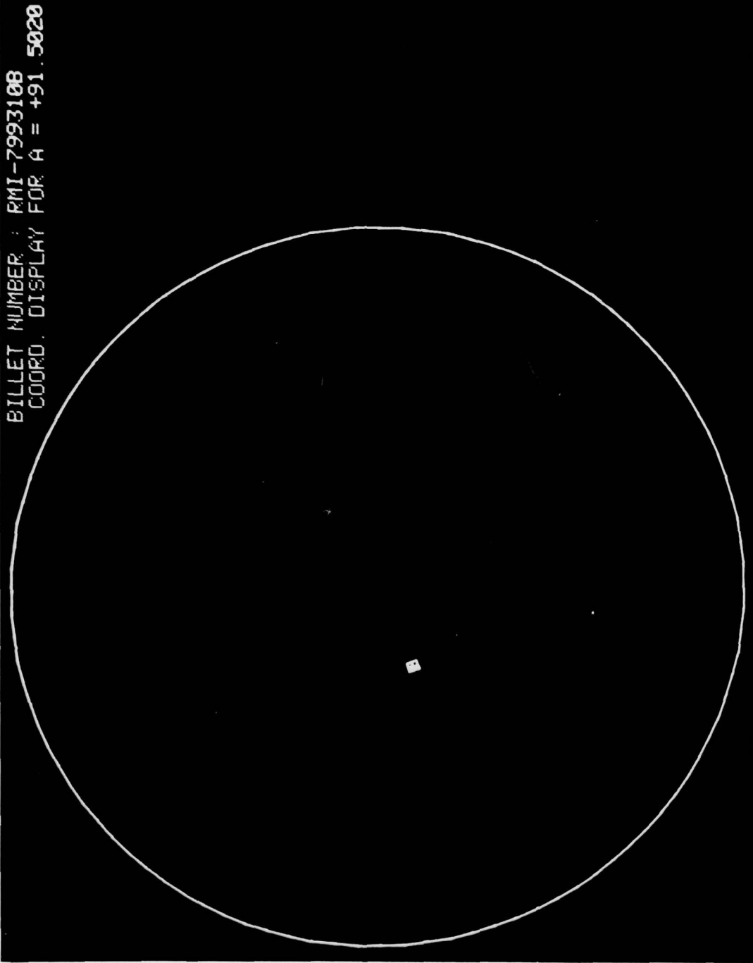
Figure 88. Defect Coordination Display (RMI-7993108, SCC = 7, R \approx \theta = A = 1 , Defect Axial Location A = 91.50-inch)
