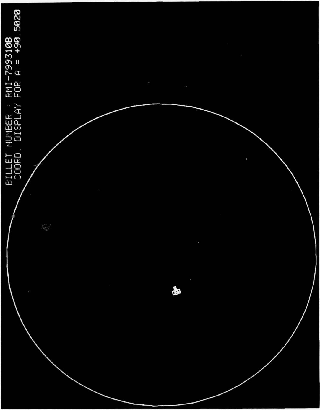
Figure 84. Defect Coordination Display (RMI-799310B, SCC = 7, R = \theta = A = 1, Billet Axial Location A = 90.50-inch)
