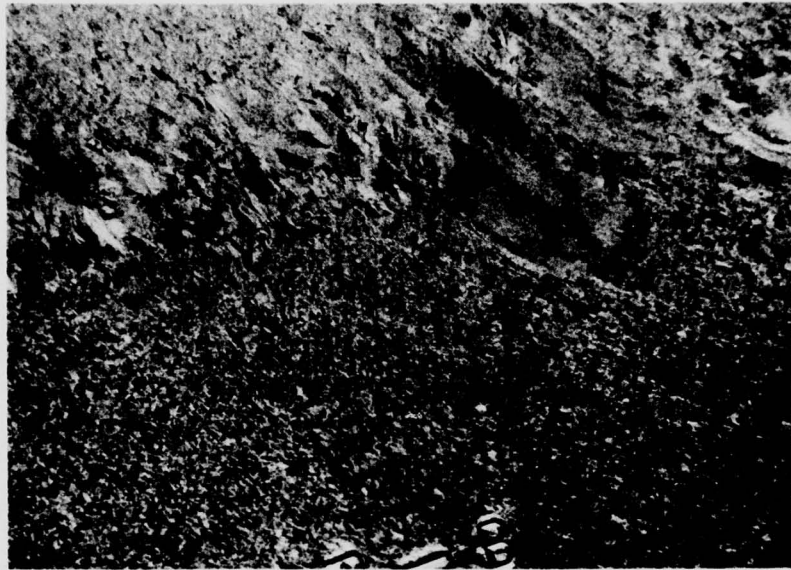
Figure 98. Grain Size Variations in 16T-B Specimen. (Approx. 4.6X)
