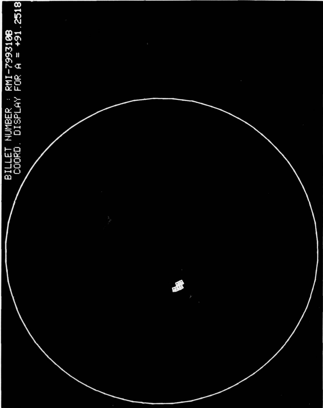
Figure 87. Defect Coordination Display (RMI-7993108, SSC=7, R=θ=A=1, Billet Axial Location A=91.25 inch).
