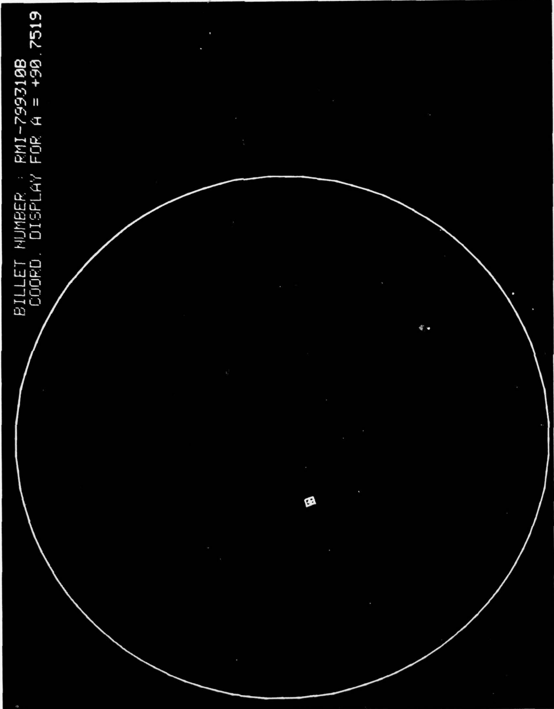
Figure 79. Defect Coordination Display (RMI-799310B, SCC = 15, R = \theta = A = 1 , Billet Location A = 90.75-inches)
