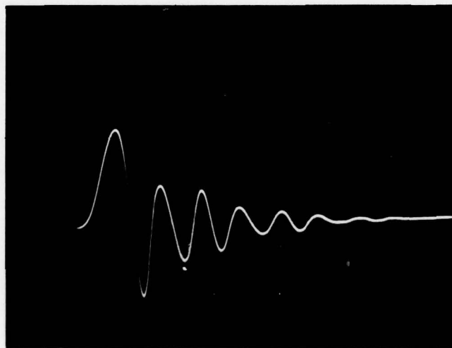
Figure 10. Pulsar Output of Component Manufacturer B 1 in Thru-Transmission Instrument Mode. (Vertical Display: 500.0 V/cm Horizontal Display: 0.1 \mu s/cm)
