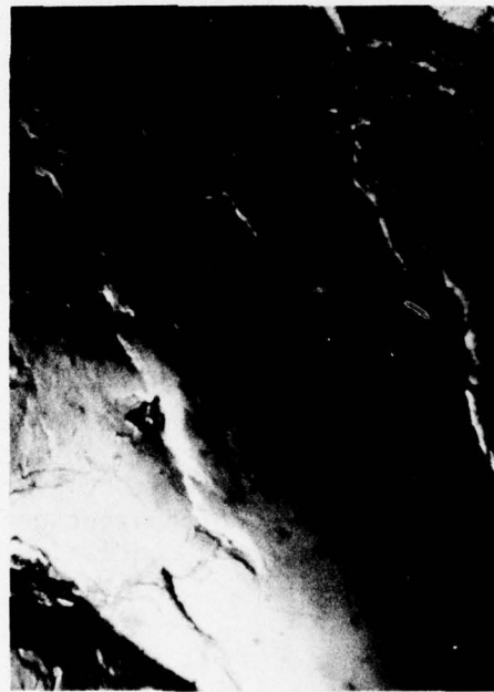
Figure 114. Fracture surface and unbond in TRW defect No. 7.
