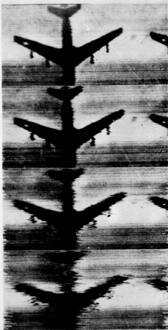
Figure 4-14 (Continued). Gaussian Line Jitter Applied to an Infrared Image of Parked Aircraft
