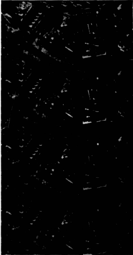
Figure 4-18. Additive Gaussian Spot Noise Applied to a Synthetic Aperture Radar Image
