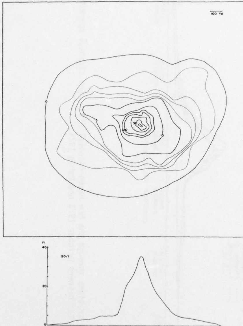
Figure 24. Contours (in ft) of the thickness of the deposit of dredged sediment at the New Haven disposal site and an east-west cross section through the center of the mound.
