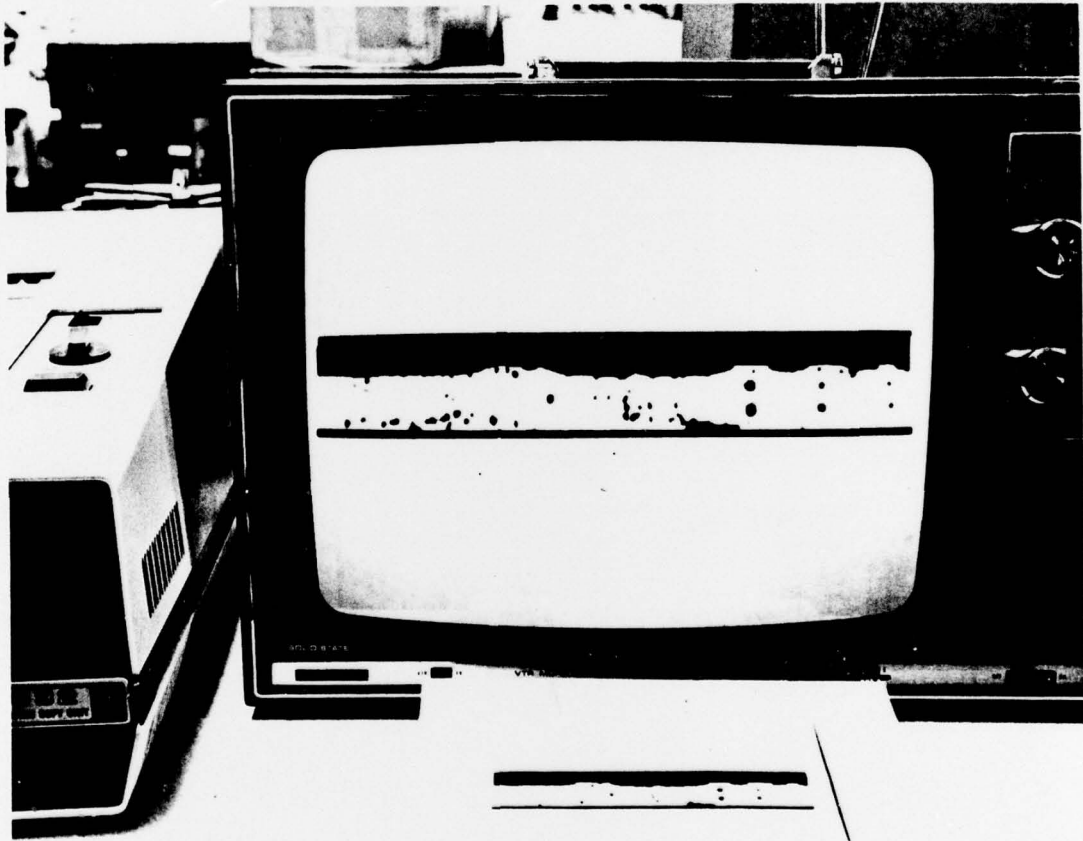
Figure 4. C-scan of brazed copper band. 19-066-1204/AMC-77
