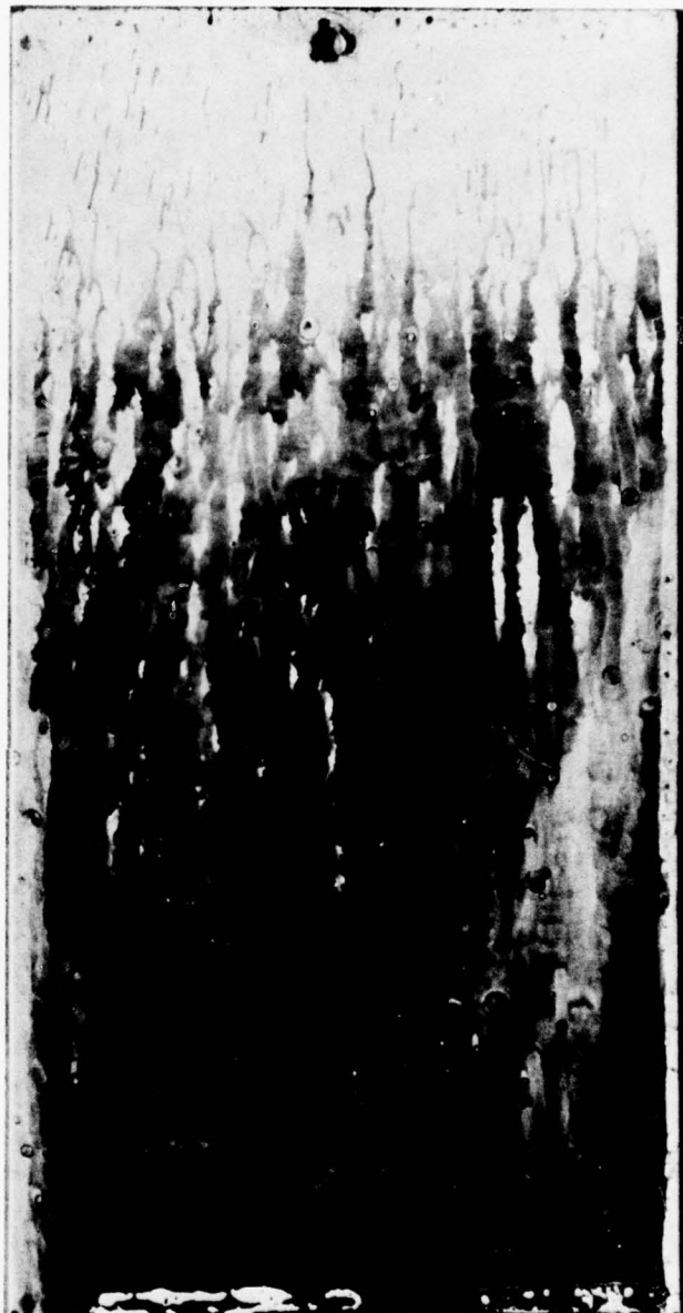
EPOXY PRIMER MIL-P-23377 TOPCOAT MIL-L-81352 WHITE OVERCOAT NRL CLEAR
