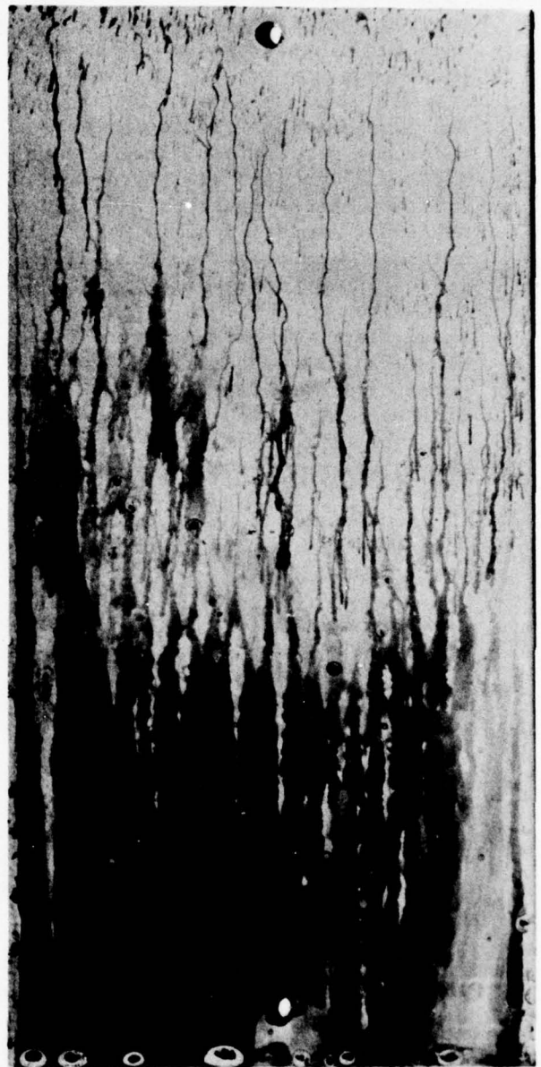
EPOXY PRIMER MIL-P-23377 TOPCOAT MIL-C-81773 GRAY OVERCOAT LOWER HALF NRL CLEAR
