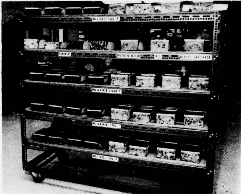
Figure 2. Movable rack. Specimens were moved in and out of coldroom in this way.
