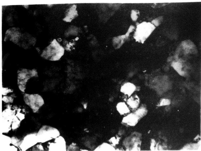
Figure 23. Electron micrograph of hydrostatically extruded Al-0.05% Fe wire. Solution treated and furnace cooled before extrusion.
