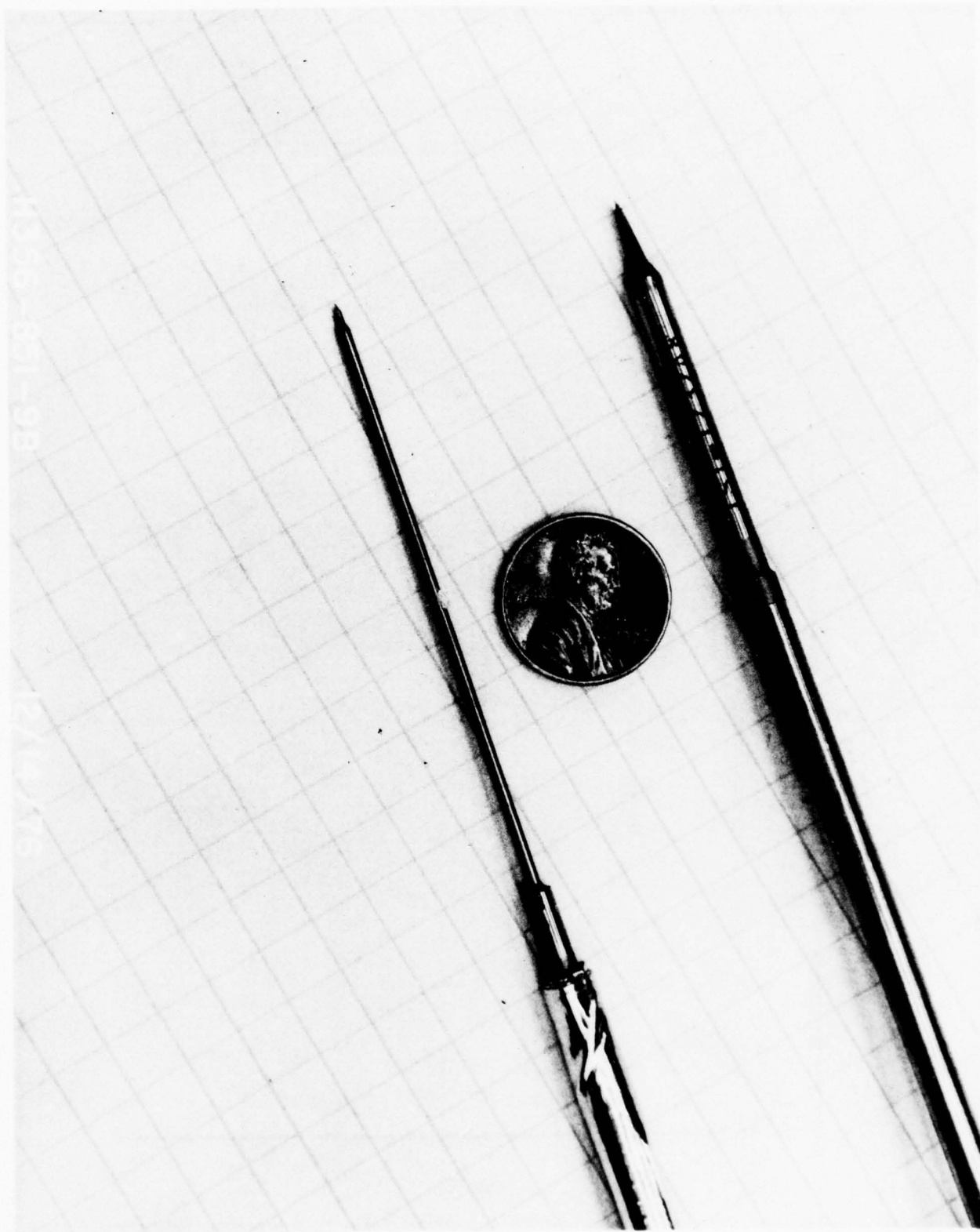
Figure A-2. Conical Hot Film Probe (Upper) and Dual Sensor Probe (Lower)
