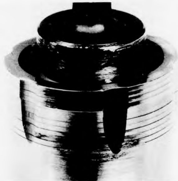
Figure 121. Spring After Task II Full-Speed Overrun Tests.
