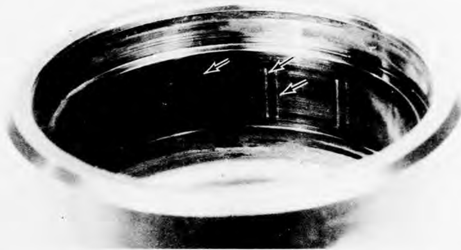
Figure 136. Ramp-Roller Clutch, Outer Housing at Completion of Task II Dynamic Load Test.
