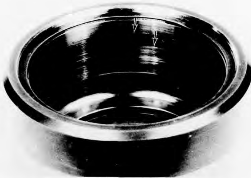
Figure 67. Ramp-Roller Clutch, Outer Housing Roller Contact Area After 5 Hours Full-Speed Overrunning, Task I.
