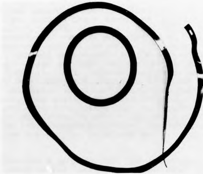
Figure 109. Oil Dam Snap Ring and Bronze Bushing, Task I Turbine Dynamic Load Test, Ramp-Roller Clutch.
