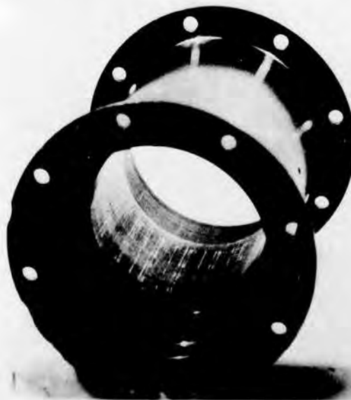
Figure 64. Sprag Clutch Outer Shaft Bore After Full-Speed Overrunning Test, Task I.
