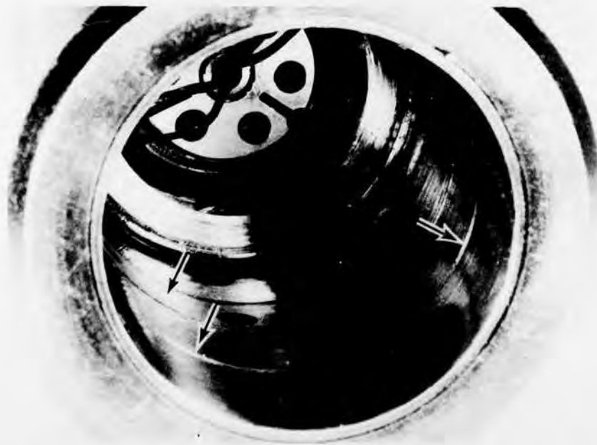
Figure 82. Spring Clutch Output Housing After 3 Hours of Differential-Speed Overrunning, Task I.
