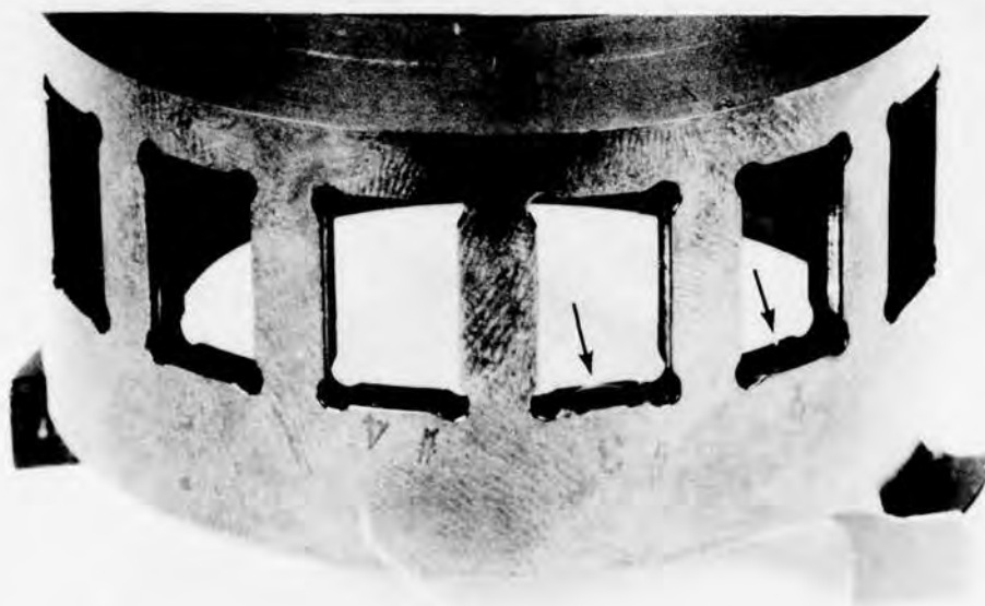
Figure 98. Roller Carrier After Differential-Speed Overrunning Test, Task I.
