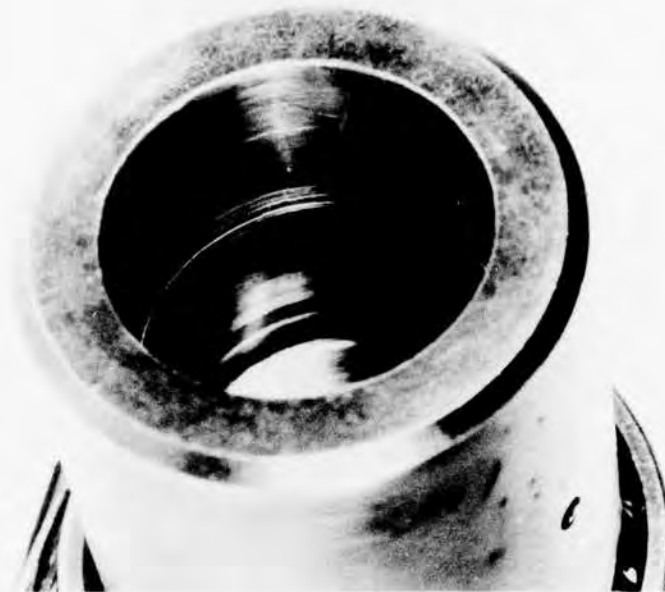
Figure 120. Spring Clutch Output Housing After Task II Full-Speed Overrun Tests.
