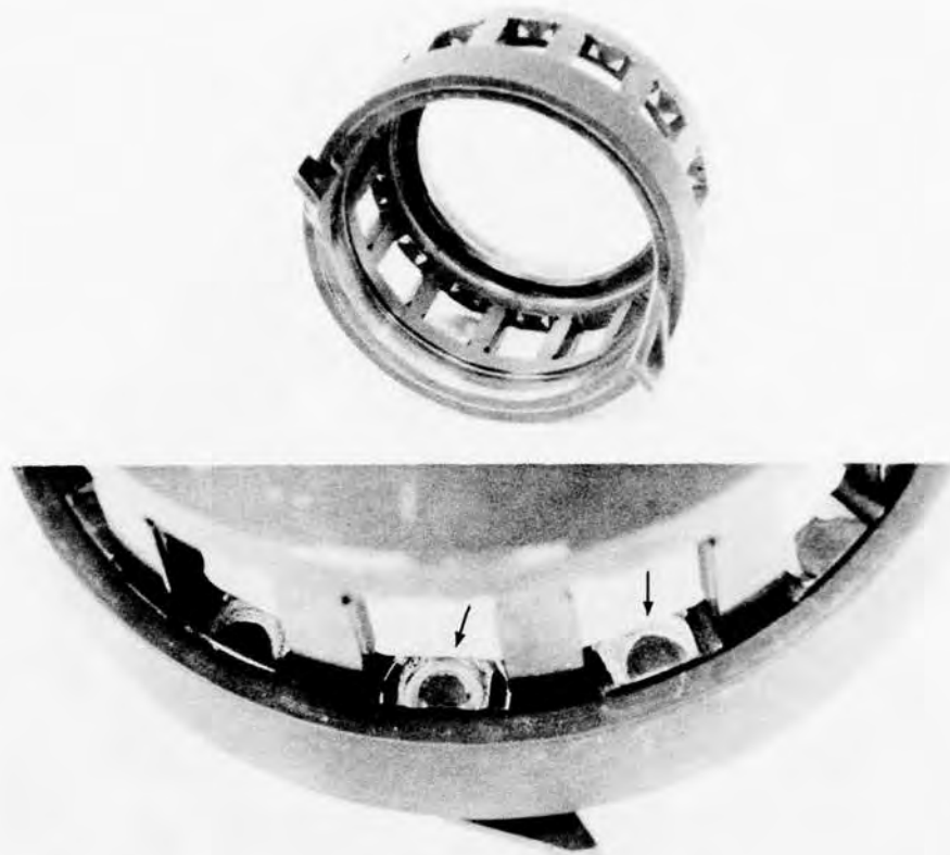
Figure 130. Roller Retention Carrier After 15 Hours, Task II Differential-Speed Overrun Test.
