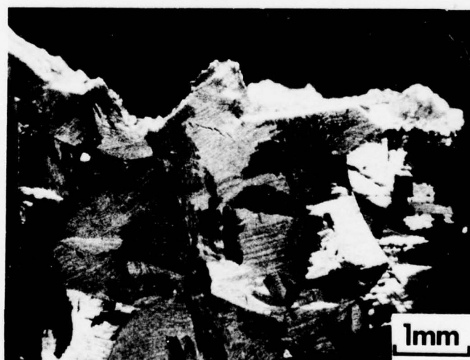
Figure 31 (a) General Appearance of the Fracture of Specimen No. 49 Tested at 400°F. The apparent fracture origin is indicated by an arrow. (b) A Longitudinal Section Along the Line Indicated in (a), Showing the prior \beta grain size adjacent to the fracture surface.
