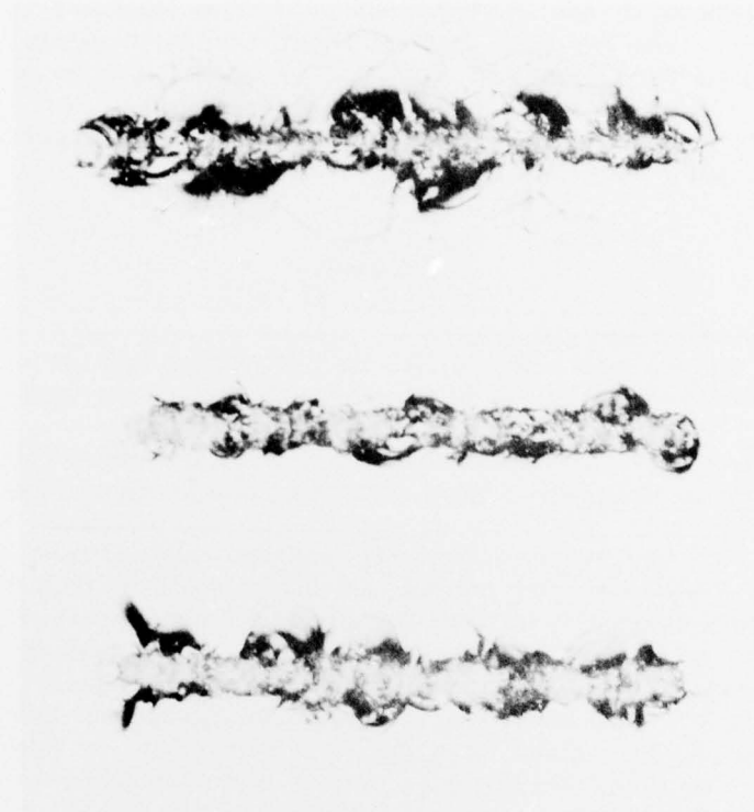
Figure 5. Characteristic scratch appearance; Upper: Chemical-tempered lens; Middle: Heat-tempered lens; Bottom: Nontempered lens.
