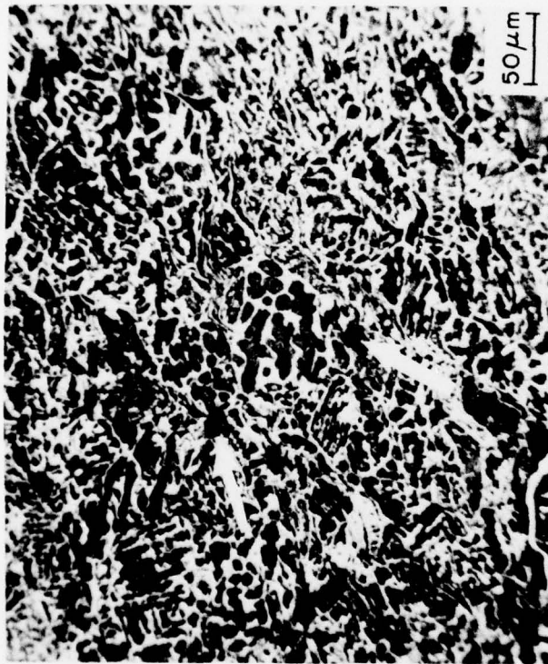
Figure 19. Microstructure of a 2.6% white cast iron compact after warm pressing at 700°C and 69 MPa for 5 hours to a final relative density of 95%. (A) shows the former ledeburite colonies dispersed in a matrix of proeutectoid cementite. The arrows point out two such colonies. (B) details the structure of one of these colonies. The structure consists of fine ferrite grains (<2 \mu m) stabilized by fine spheroidized cementite particles (<1 \mu m).
