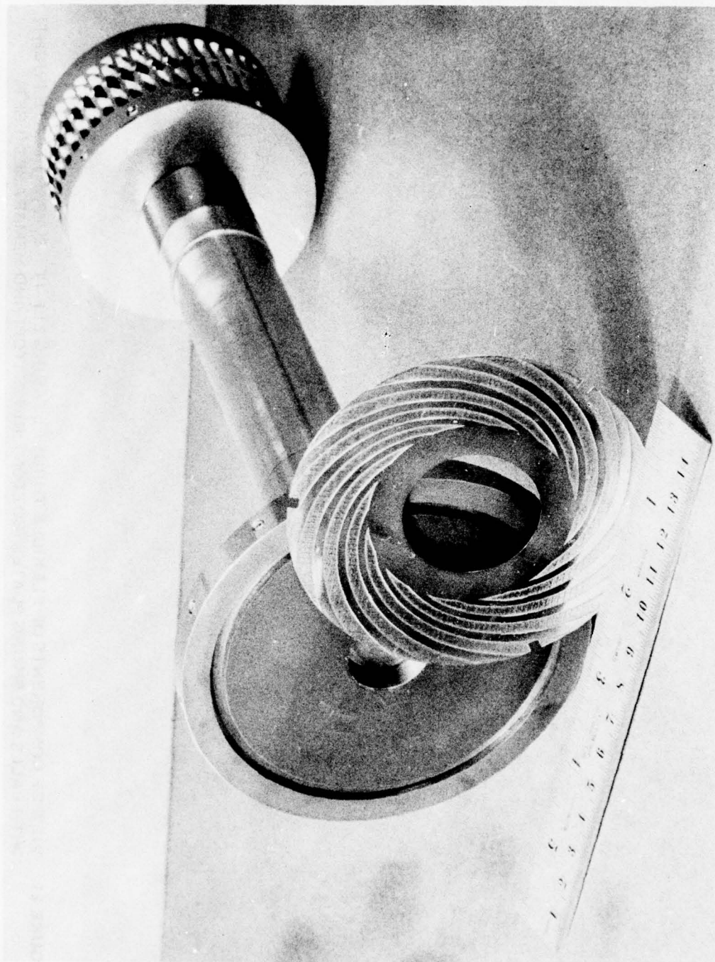
FIGURE 22. END VIEW OF ROTOR ASSEMBLY, SHOWING \text{Cr}_2\text{O}_3 -PLATED RUNNER AND SPIRALLY GROOVED MEMBRANE
