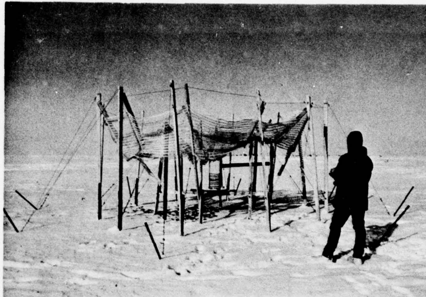
Figure 6. Wyoming snow gauge.
