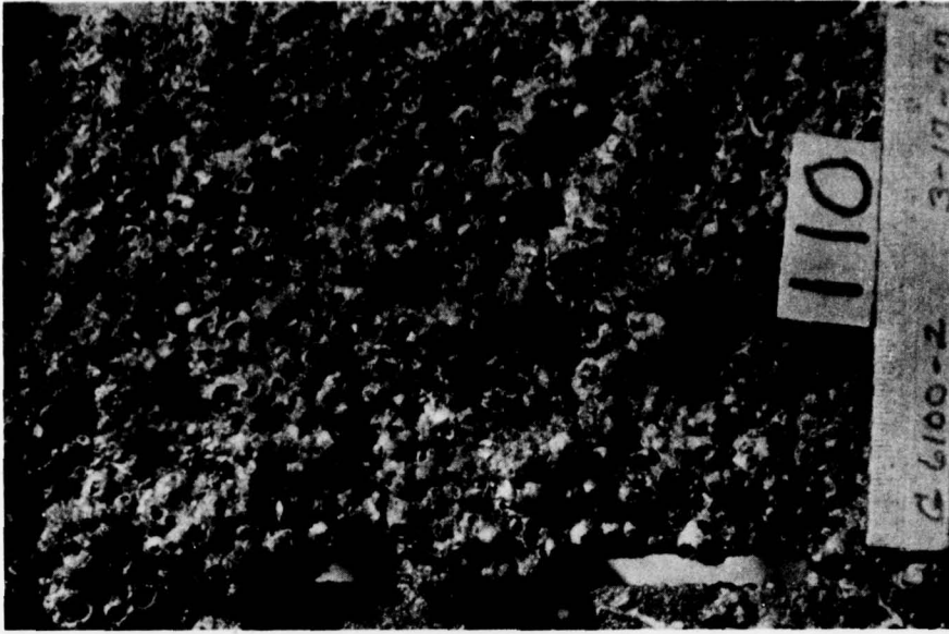
Panel No. 110 ----- Uncoated Steel Control Panel
