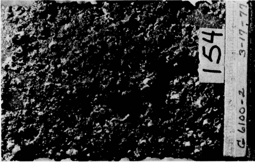
Panel No. 154 System No. CG-36 Acrylic-Organometallic Toxic Polymer on Plastic
