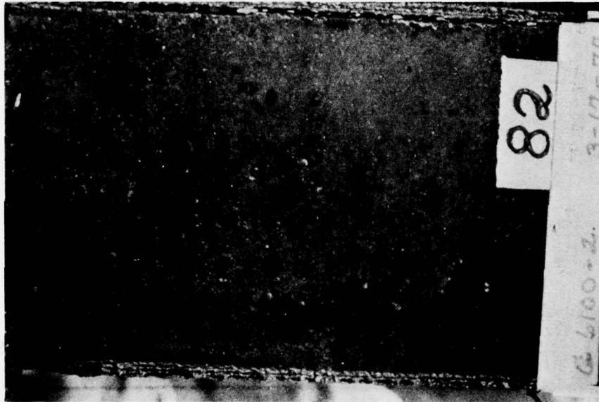
Panel No. 82 System No. CG-20 Elastomeric Sheet With Organotin Toxicant on Steel
